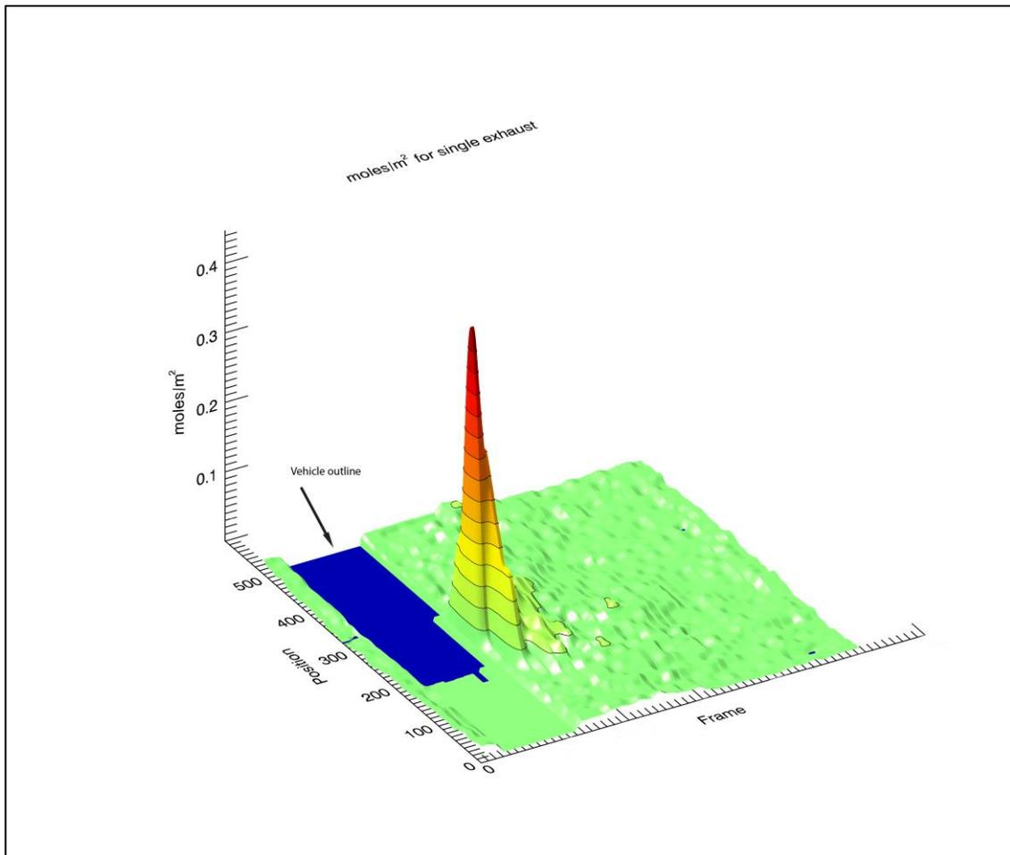
The gram per mile is calculated on the first few frames after the vehicle has passed while concentrations are relatively high and only in the neighborhood of the tailpipe. This mitigates any effects of interfering plumes of vehicles in the vicinity.
