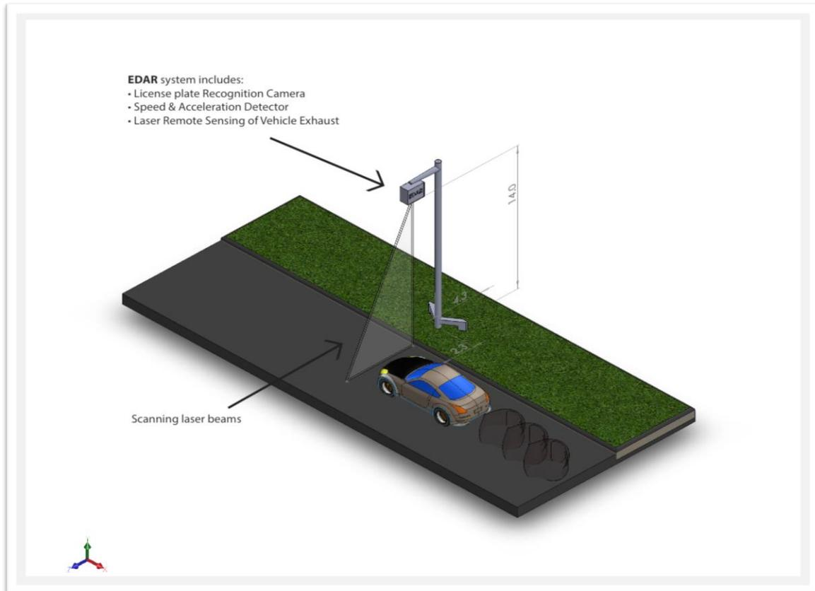
The gas sensor emits a sheet of invisible laser light from above that can unambiguously measure specified molecules emitted from any vehicle that breaks the beam. The lasers are tuned for the pollutants CO<sub>2</sub>, CO, NO, and HC. Due to the fact that the gas sensor looks down from above
