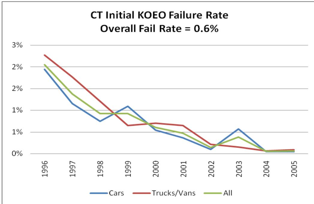
This chart shows failure rates by model year for the Key-On Engine Off (KOEO) test, which is part of the OBD test. The average KOEO failure rate for all vehicles was 0.6%. The KOEO determines if the MIL bulb is working. The bulb should illuminate when the key is turned to the on position but the engine is not started.
