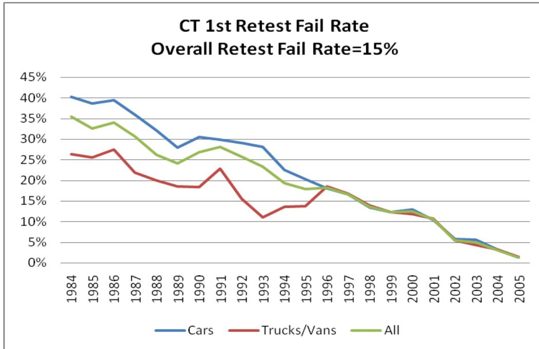
This chart shows the percent of vehicles by model year that fail their first retest. The failure rate is highest for the older vehicles, which is typical of most programs. Overall, about 15% of the vehicles fail their first retest.
