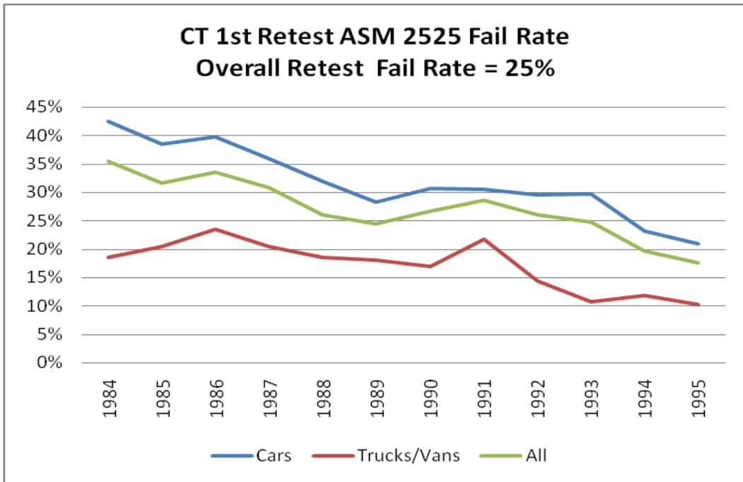
This chart shows the percent of vehicles by model year that fail their first ASM2525 retest. The retest failure rate generally is highest for the older vehicles. Overall, 25% of the vehicles fail the first ASM2525 retest. There were too few 1996+ vehicles receiving ASM2525 retests for a meaningful analysis.
