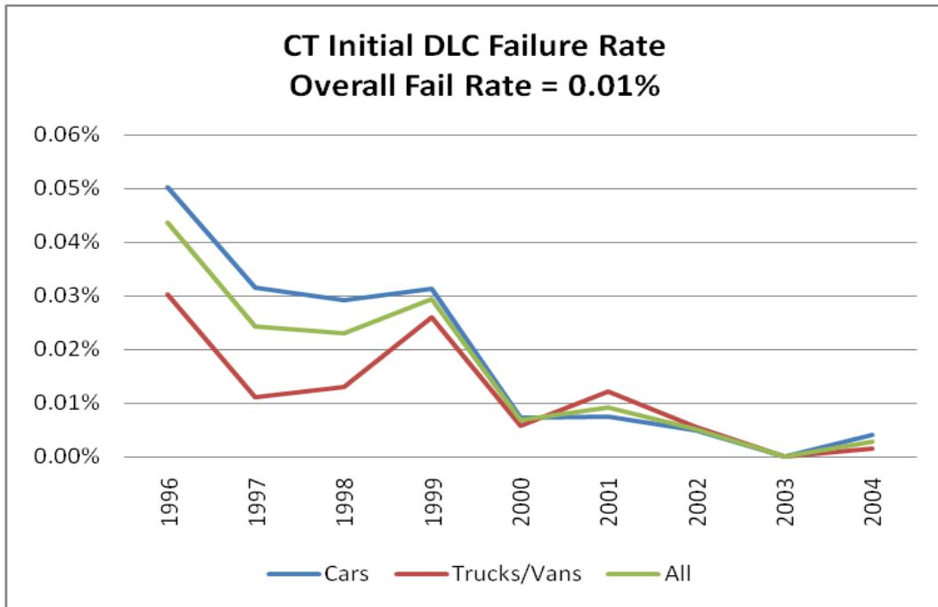
This chart shows the percentage of vehicles that fail because the OBDII connector, termed DLC, is missing, damaged or obstructed. Overall, 0.01% of the vehicles fail for this reason.
