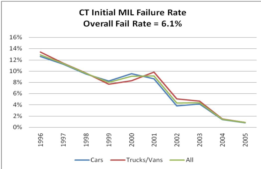
This chart shows the percentage of vehicles that fail the MIL Command check that's part of the OBD test. Most OBDII failures are for the MIL Command check. The average MIL failure rate for all vehicles was 6.1%. This graph shows that older vehicles have a higher failure rate, as expected.
