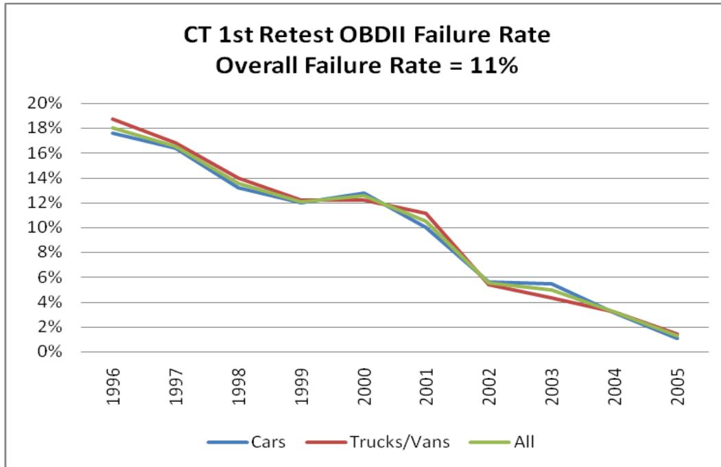
This chart shows failure rates by model year for the first OBD retest. The average failure rate for all vehicles in the first OBD retest was 11.0%. Note that Connecticut requires OBD failures to meet readiness requirements when retested. If a vehicle does not meet readiness requirements when retested, the inspection is aborted. Vehicles that are not ready on retest are not included in the above fail percentage.
