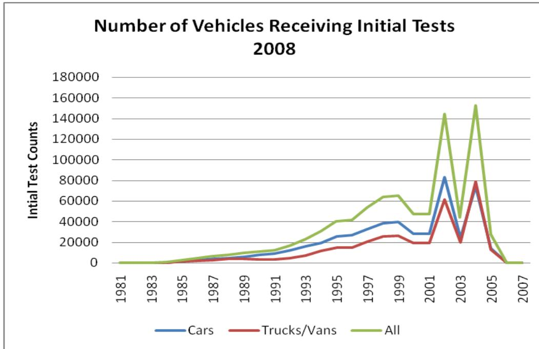
This chart shows the total number of inspections by model year and vehicle type. The first four model years are exempted from testing, so the number drops sharply for 2005 and newer model years.
