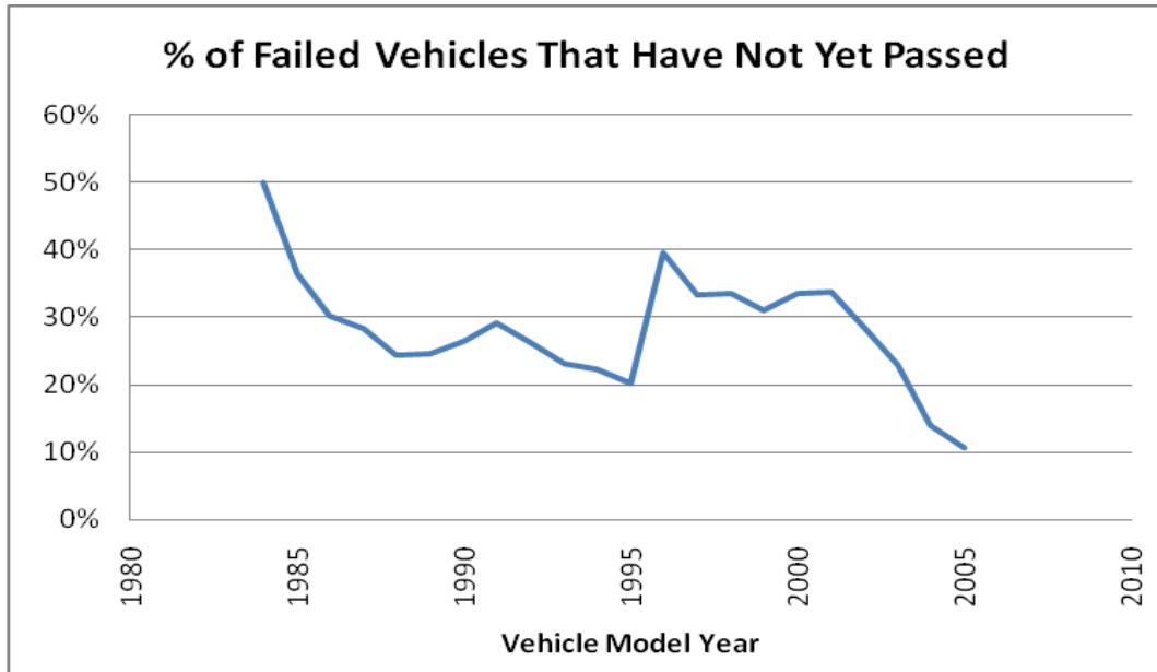
This chart shows the percentage of vehicles that fail the emission test in the first three months of 2008 that never ultimately passed in 2008. The increase from 1995 to 1996 indicates that compliance with the OBD test may be more difficult than the tailpipe test used for pre-1996 vehicles.
