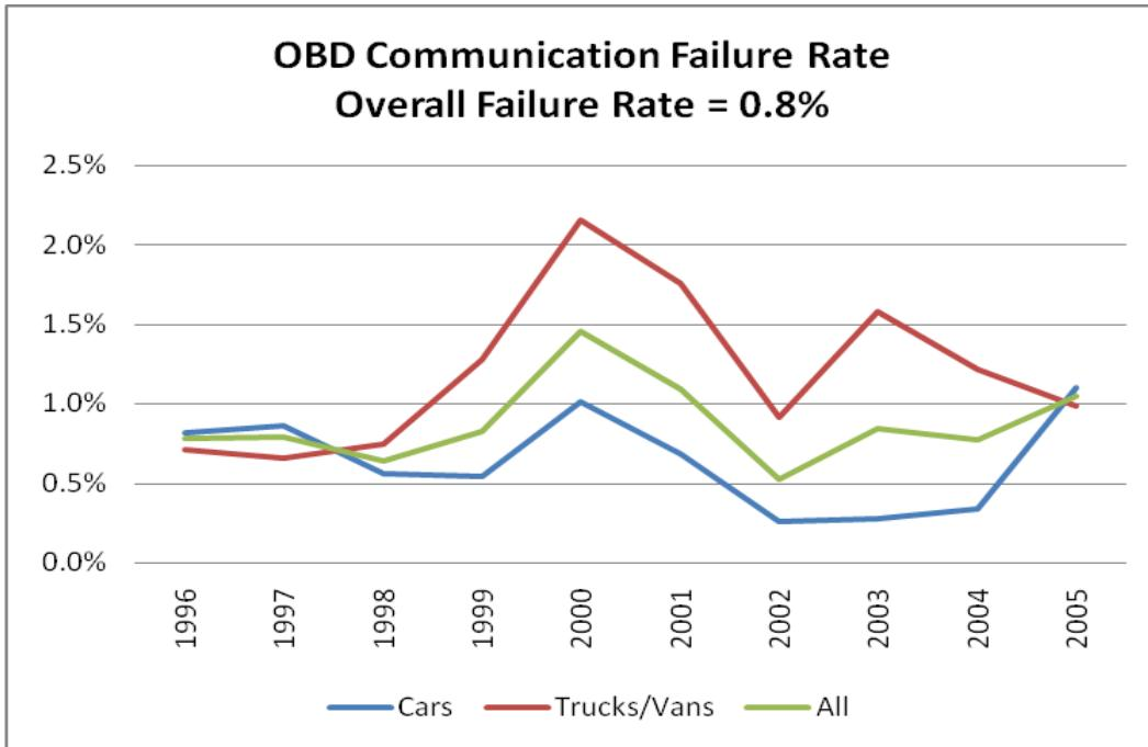
This chart shows the percentage of vehicles that fail to communicate with the OBDII test equipment. Overall, 0.8% of the vehicles fail for this reason. Vehicles with known communication problems receive ASM tests instead of OBDII tests.
