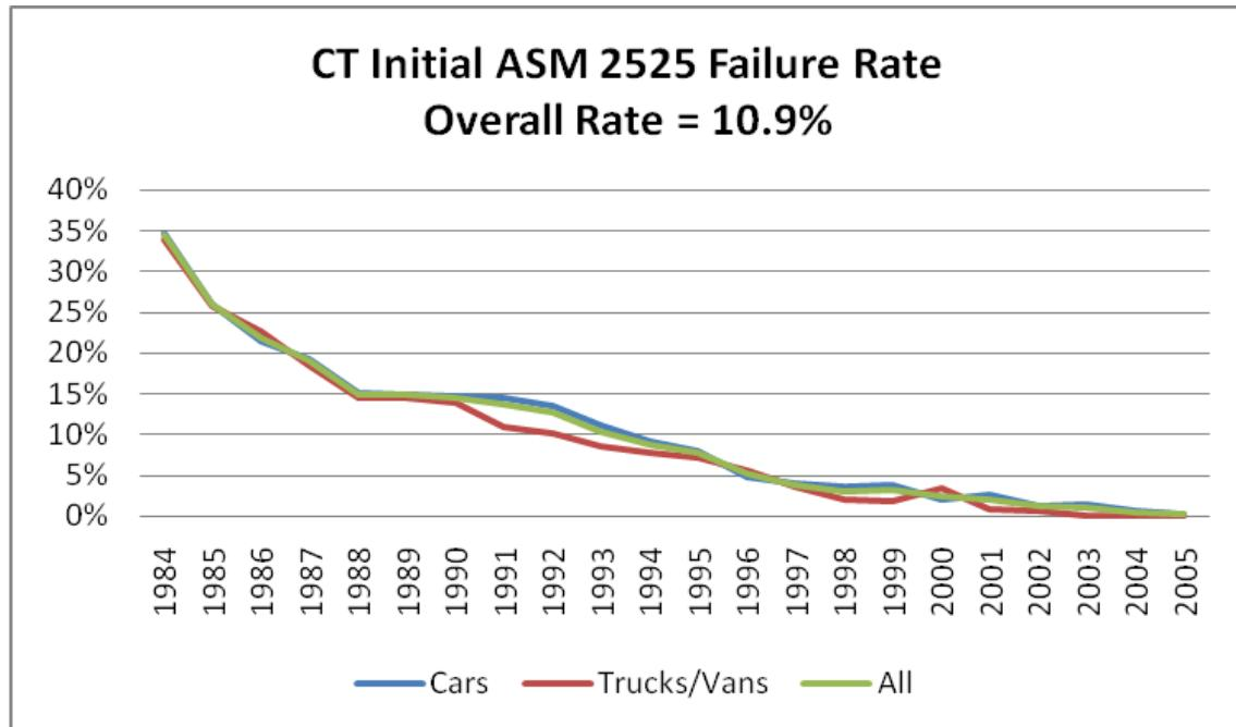
This chart shows failure rates by model year for the ASM2525 test. The average ASM2525 test failure rate for all vehicles was 10.9%. Typically, a higher failure rate for older model year vehicles is expected.
