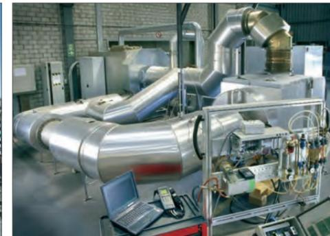
In-house test bed for filters and regeneration systems
