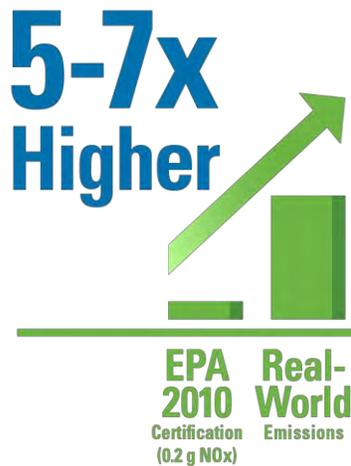
Heavy-duty drayage trucks: Diesel trucks tested in study exceed certification level
