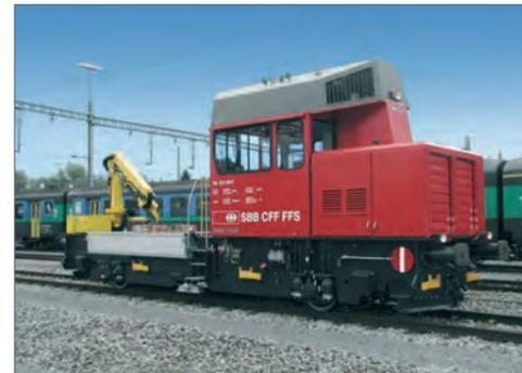
Tm234, 550 KW with soot particle filter and DeNOx
