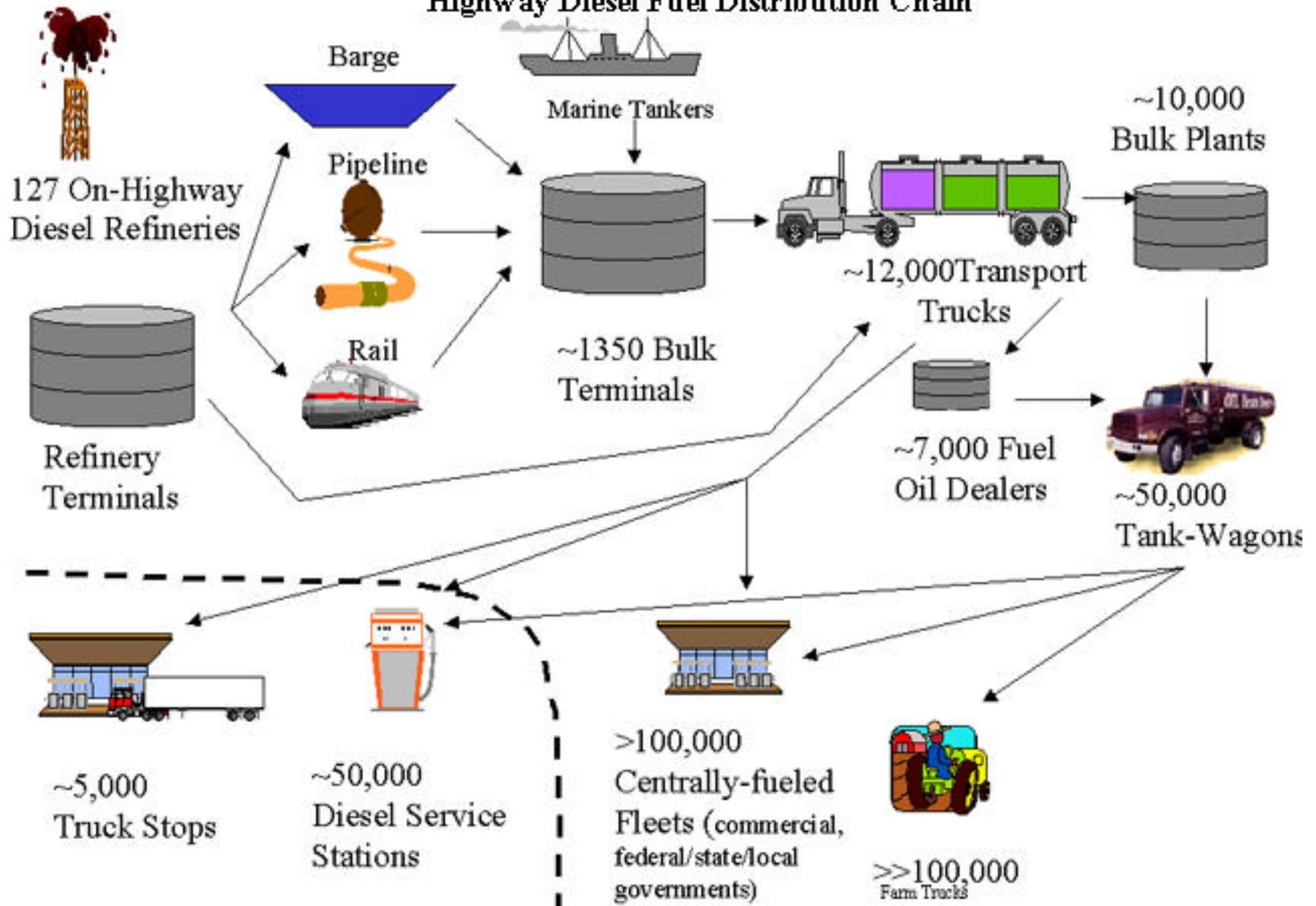
foreign countries, for example. In cases where pipeline service is limited, fuel is also shipped to the terminal by rail car.
