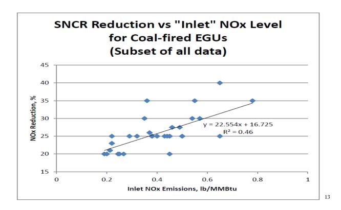
Using the  $50^{th}$  percentile  $NO_x$  baseline of 0.135 lb/MMBtu and the regression equation provided in the figure above, I obtain a  $NO_x$  reduction efficiency of 19.8%. Using the  $95^{th}$  percentile  $NO_x$  baseline value of 0.157 lb/MMBtu, the estimated SNCR efficiency is 20.3%.
