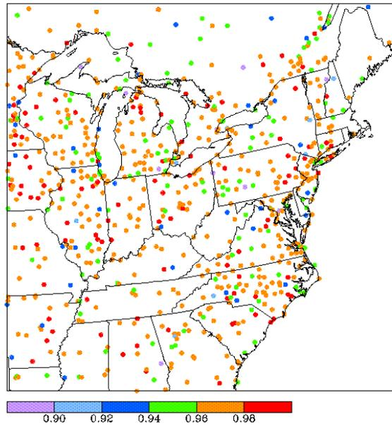
Figure 5b: Spatial distribution of correlation coefficients for Temperature between MM5 and NWS data for winter months – January to March, 2002 (top panel), and summer months - May to September, 2002 (bottom panel).
