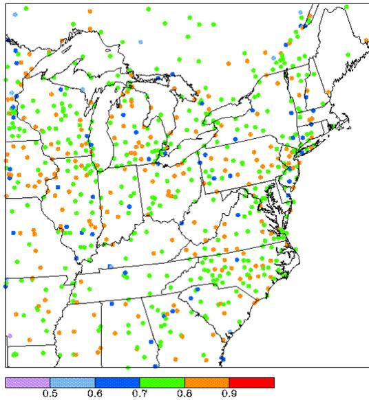
Figure 5a: Spatial correlation estimates between MM5 and NWS data for wind speed for winter months – January to March, 2002 (top panel) and summer months - May to September, 2002 (bottom panel).
