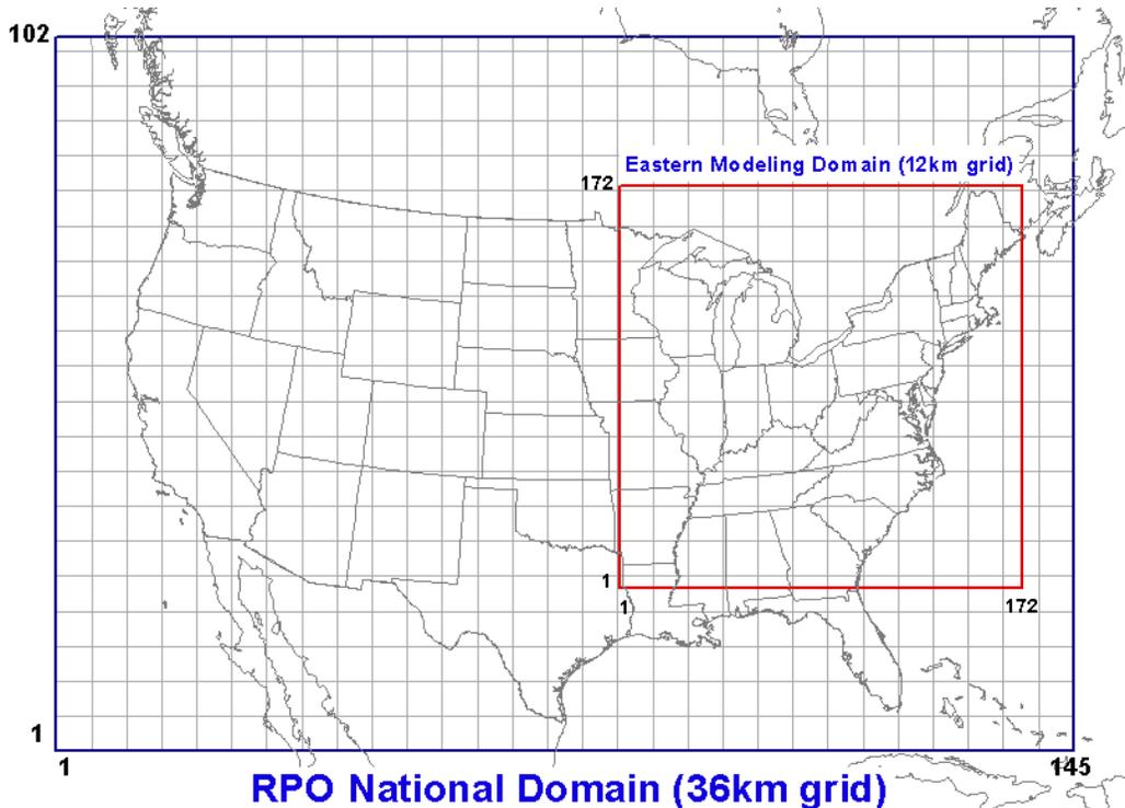
Figure note: Outer (blue) domain is a 36 km grid and inner (red) domain is a 12 km grid. The gridlines are shown at 180 km intervals (5 × 5 36 km cells/15 × 15 12 km cells).
