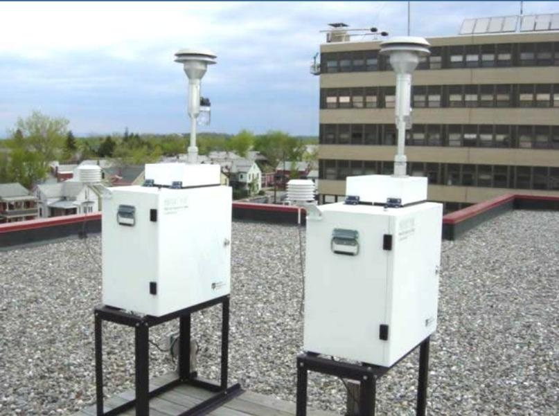
DEEP operates 9 PM2.5 FRM (filter based) sites in the air monitoring network using Thermo Partisol®-Plus 2025/2025i sequential air samplers. Two of the sites, Criscuolo Park in New Haven and McAuliffe Park in East Hartford, operate on a daily sample schedule while all the other sites operate on a 1-in-3 day sample schedule.
