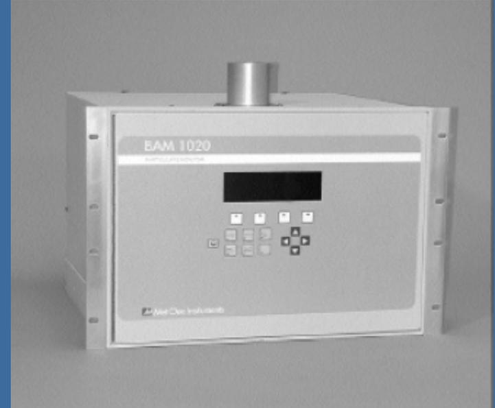
DEEP operates eleven continuous PM monitors at nine sites. This network includes continuous MetOne BAM 1020PM2.5 samplers at each of the nine sites, and paired continuous MetOne 1020 BAM PM10/ PM10-2.5 samplers at the two Ncore sites (New Haven and Cornwall). All BAM monitors are operated year-round and the hourly data is reported to AQS and is used for air quality index (AQI) reporting
