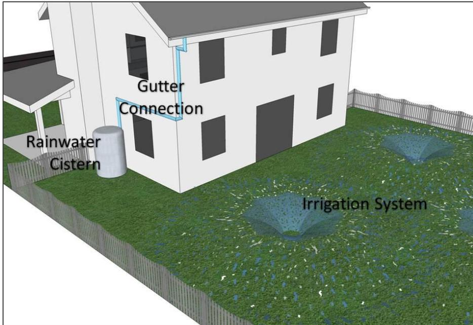
**Figure 15:** Rainwater harvesting cistern installed behind a house
