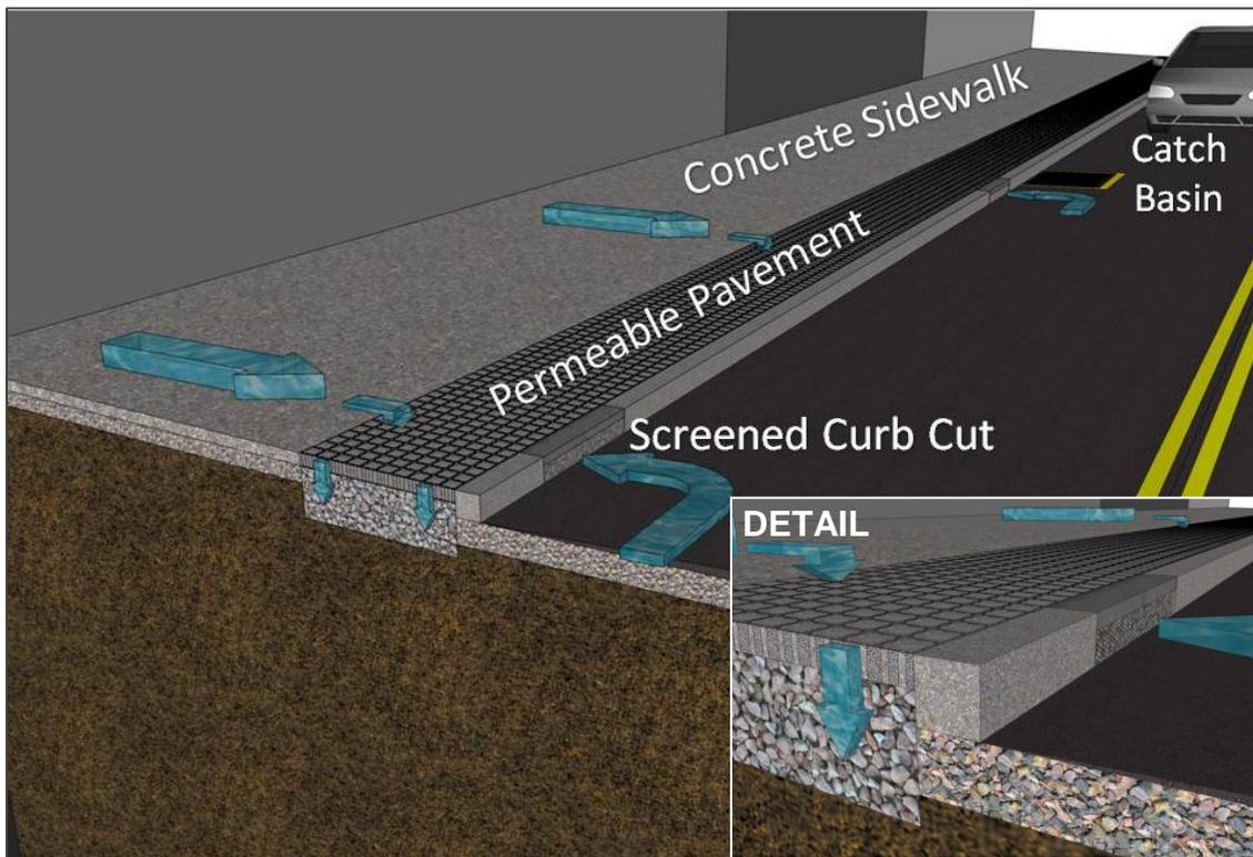
**Figure 18:** Existing sidewalk configuration (top) and proposed permeable pavement retrofit (bottom)
