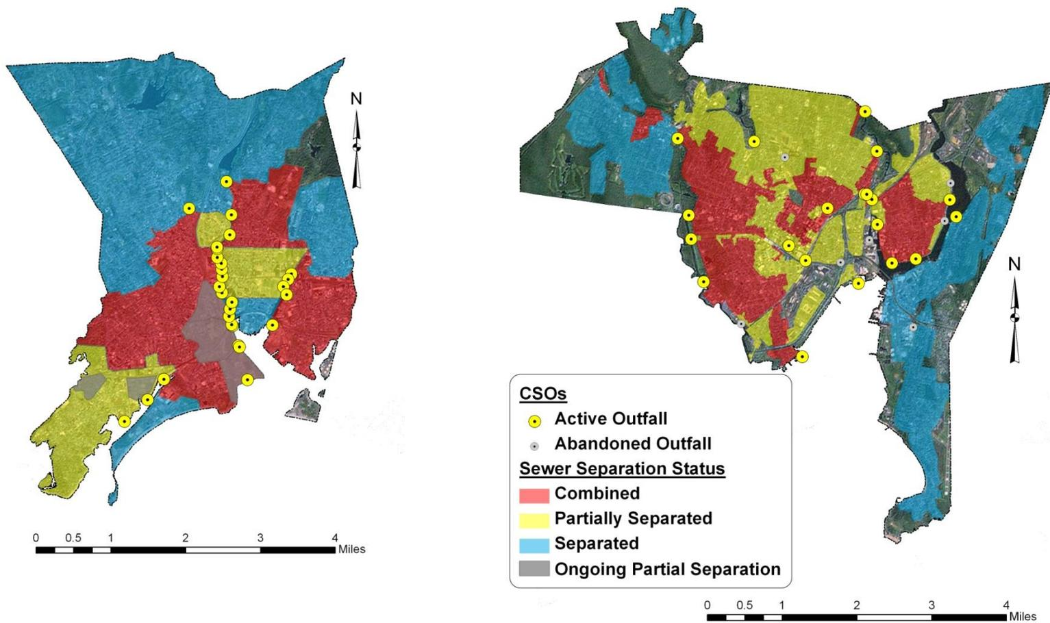
**Figure 1:** Approximate regions of combined, separated, and partially separated sewers in Bridgeport (left) and New Haven (right)
