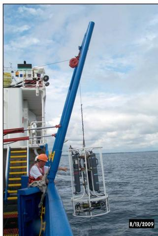
*CTD (conductivity/temperature/depth) monitoring array is deployed from OSV Bold*
