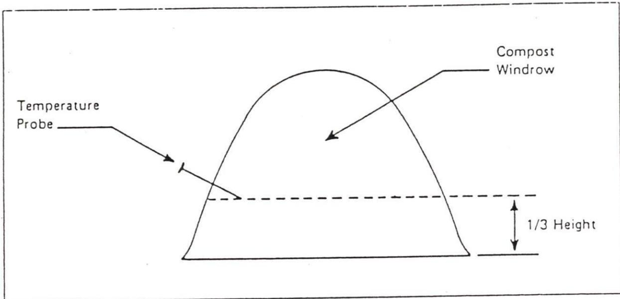
By keeping records of the temperature inside the windrows, the operator can see a trend or a general rate at which the decomposition process is moving.
