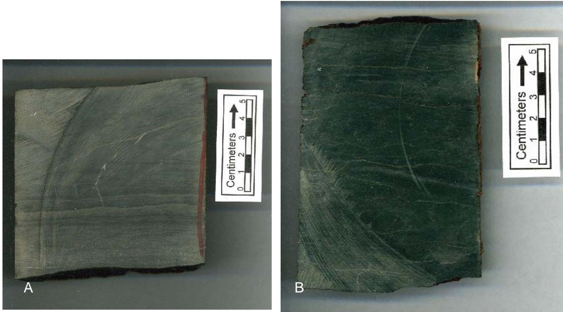
Figure 5. Perennial lake facies include laminated black shale (left), and structureless black shale (right). These samples are the Jurassic Portland Formation from the Park River Tunnel Core FD 30-T, Hartford, CT.
