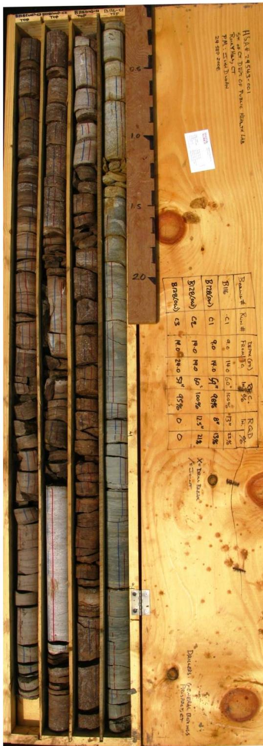
Figure 19. BH117 is in right hand compartment (see description on Figure 5). BH 123 is in two left hand compartments (see description on Figure 10). Scale is 2 ft in length and has 0.1 ft subdivisions
