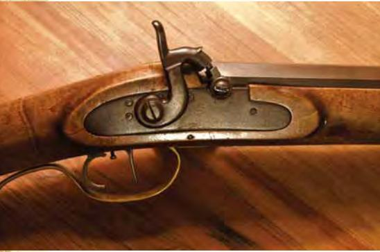
Frustrated with the relatively slow firing of the flintlock gun while duck hunting, Reverend Alexander Forsyth, a Scottish Presbyterian minister, invented the percussion cap in 1807. The percussion system uses a tiny copper or brass cup filled with a detonating compound that the shooter places on a nipple to fire the powder charge.
