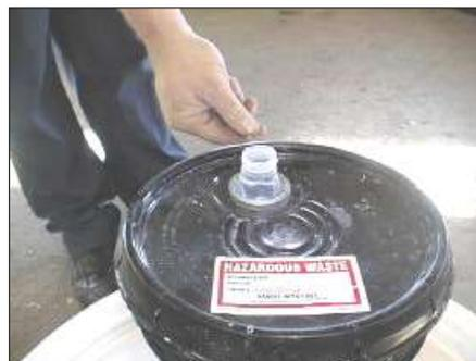
Proper storage of mercury switches
