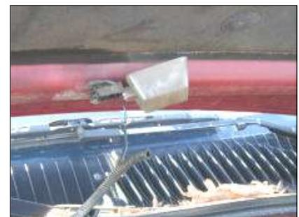
Hood light fixture with mercury switch assembly
