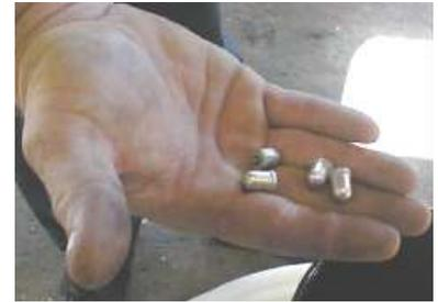
Mercury switches removed from vehicle light assemblies
