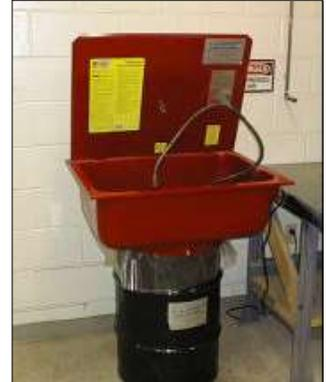
**Cold Cleaning Solvent Parts Washer
