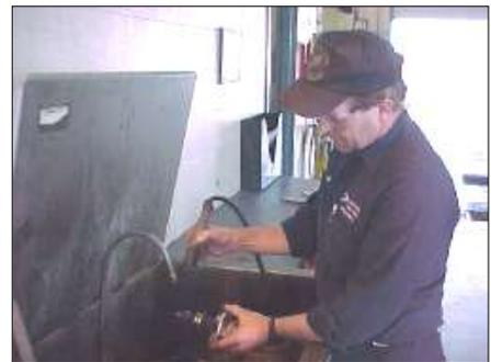
Using an aqueous-based parts washer
