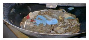
Biological materials are reacted under heat and pressure with concentrated alkali (50% sodium hydroxide), reducing the proteins to a sterile amino acid soup.
