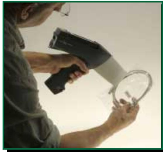
Using the XRF analyzer to test a sample
