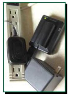
as a "wart"). The "wart" converts AC, or alternating current (the kind sent over high-voltage lines) into low-voltage DC or direct current (the kind we use for electronic circuits). Touch the wart and you can feel the heat that is wasted in this conversion. The problem with these power supplies (also called transformers) is that by design they are very inefficient and power conversion is always taking place, even when the appliance is not being used.
