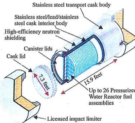
Left: diagram of transport cask with canister.
