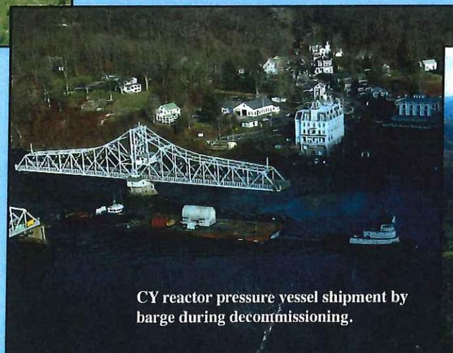
CY reactor pressure vessel shipment by barge during decommissioning.
