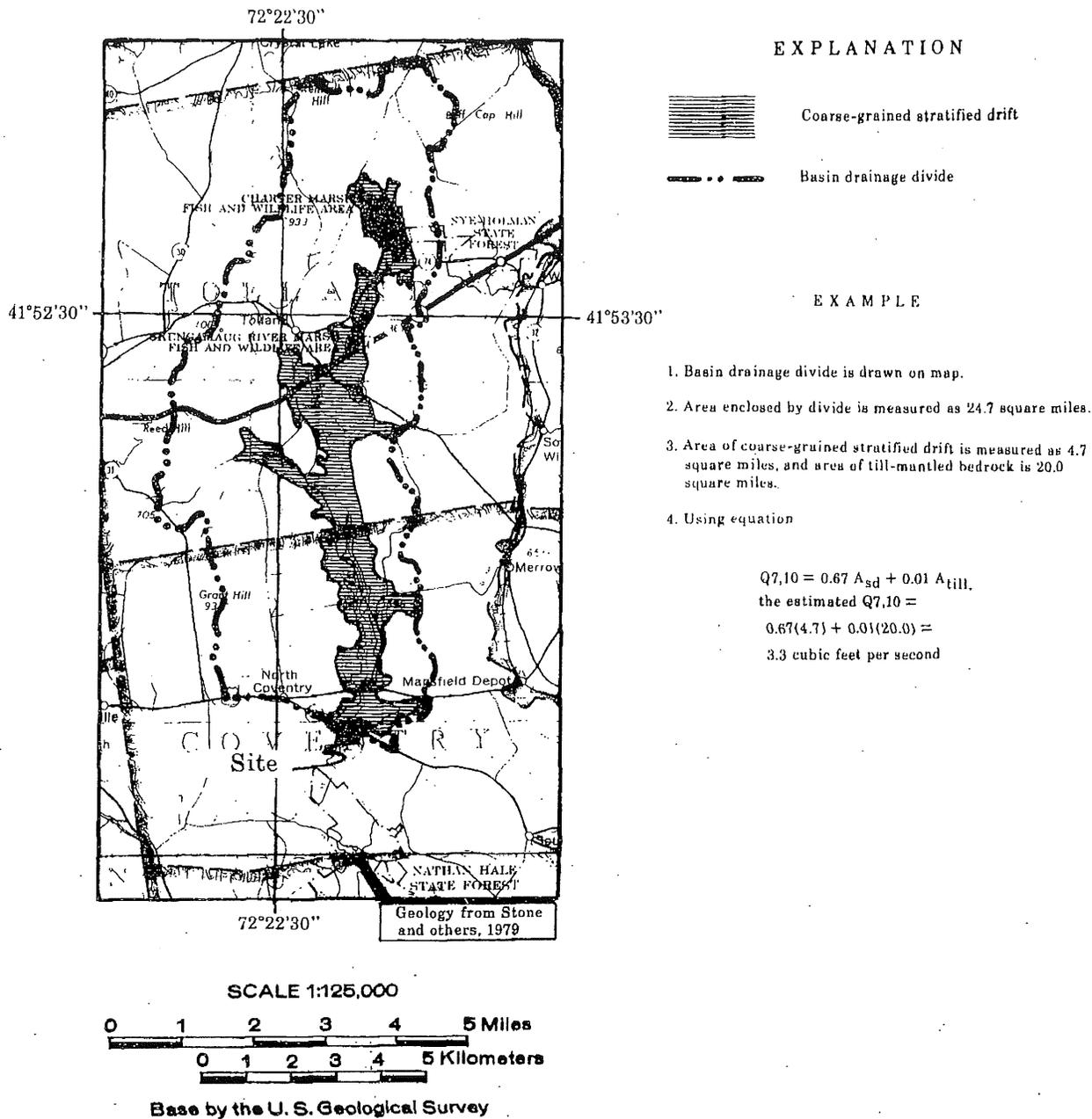
Figure 6.--Method of estimating the 7-day, 10-year low flow at an ungaged site
