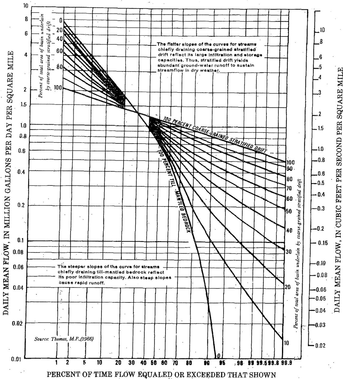
Figure 3.--Regional duration curves showing effects of basin geology on streamflow
