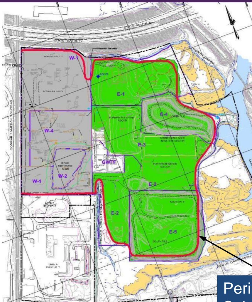
Perimeter Subsurface Hydraulic Barrier Wall
