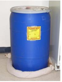
should be able to contain the volume of the largest container or 10% of the volume of all containers in storage, whichever is greater.
