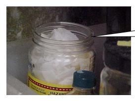
Waste Container in a Satellite Accumulation Area
