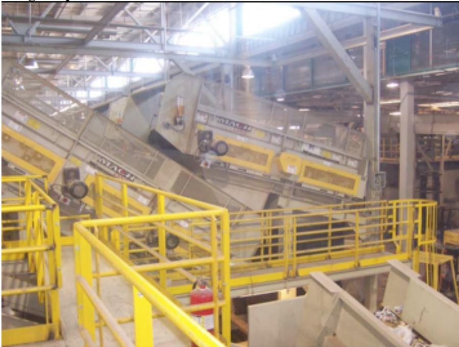
**One of Two 3-Way Polishing Screens Separating 2" Minus Fines, 3 Dimensional Items (Containers), and 2-Dimensional Items (Paper and Plastic Film). Screen in Back of Photo.**
