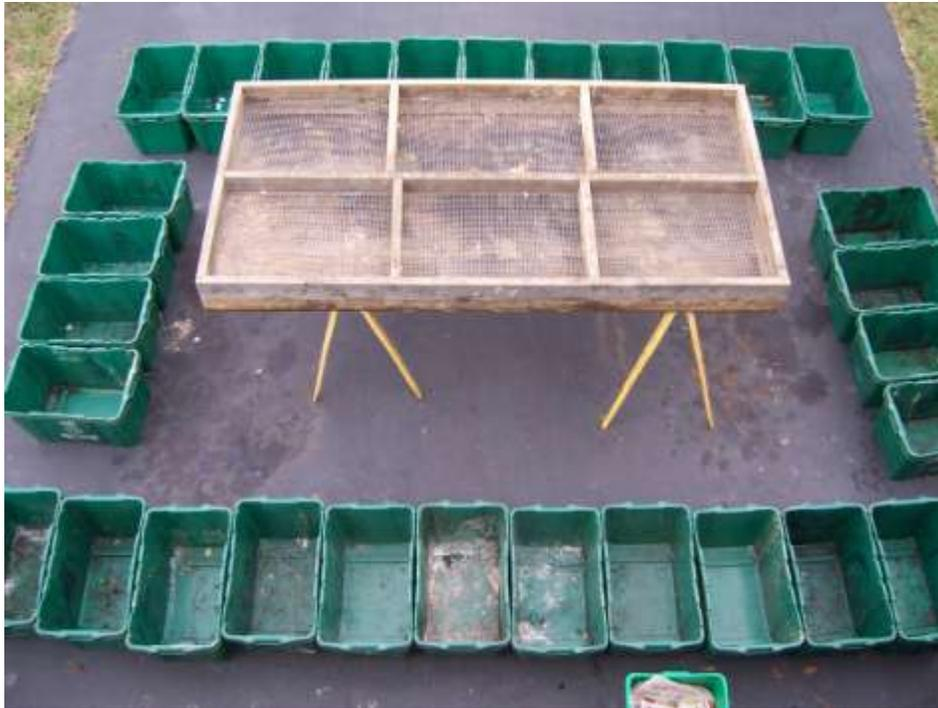
Once the sample has been acquired and placed on the sorting table, the material will be sorted by hand into the prescribed component categories. Plastic 20-gallon bins with sealed bottoms will be used to contain the separated components. The sorting crew members typically specialize in groups of materials, such as papers or plastics.
