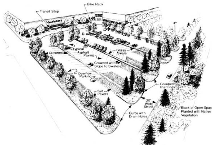
Figure 6.4.16 – Parking lot with islands attractively integrated. Source: Adapted from Connecticut, 2004.
