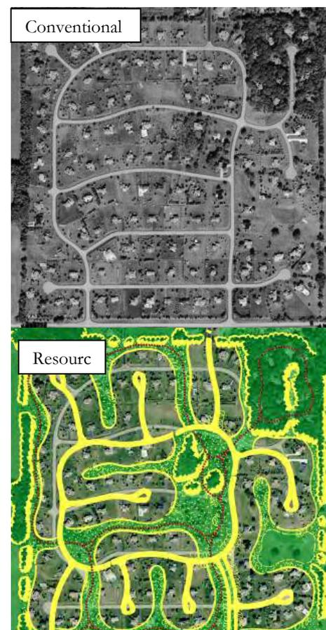
Figure 6.2.4 – integration of resource conservation into a conventional design.
