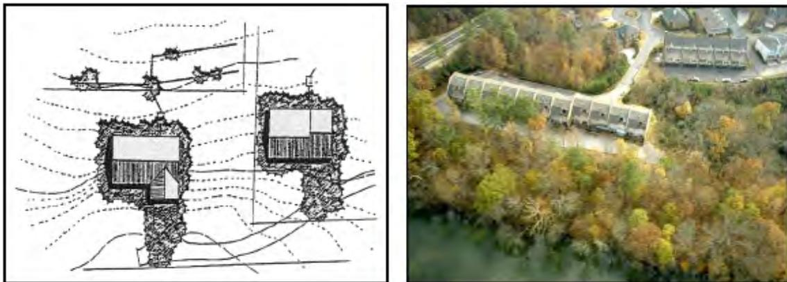
Figure 6.4.1 - Reduced limits of disturbance minimize water quality impacts. Source: Adapted from Atlanta Regional Commission, 2001.
