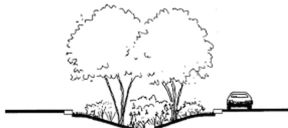
Figure 6.4.10 – Cul-de-sac infiltration island accepts stormwater from surrounding pavement. Note flat curb. Source: Adapted from Connecticut, 2004.
