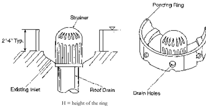
Figure 6.4.24 – Roof ponding rings. Source: Adapted from Tourbier, 1974.
