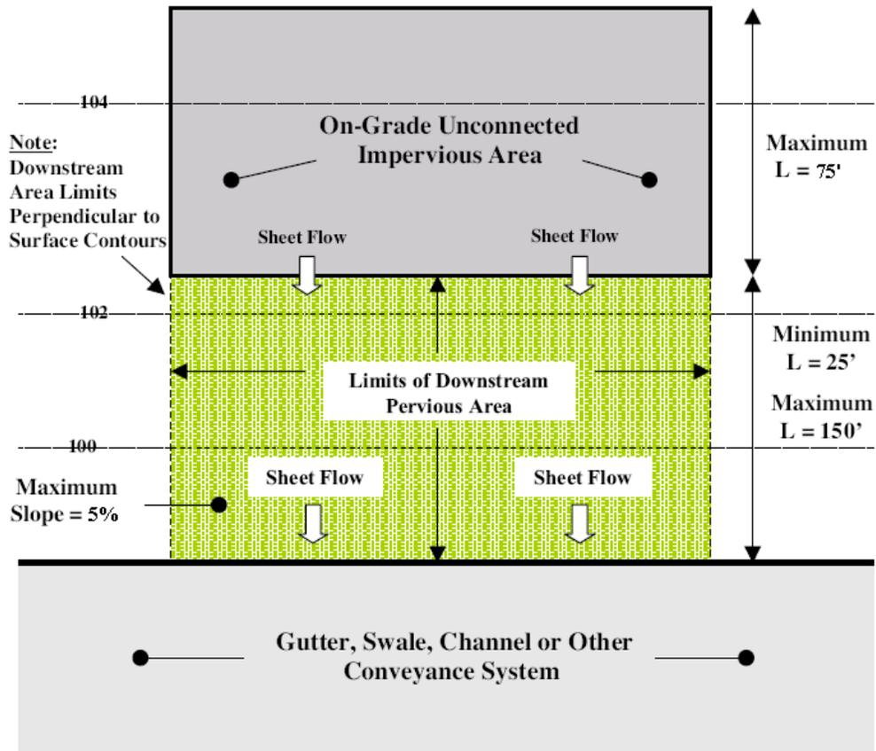
Figure 6.4.18 – Standards for disconnecting impervious surface via sheet flow. Source: Adapted from New Jersey Department of Environmental Protection, 2004.
