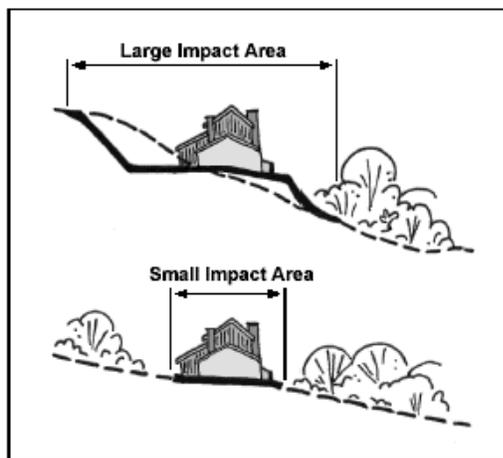
Figure 6.4.6 – Building on flatter slopes reduces the impact of development. Source: Adapted from Atlanta Regional Commission, 2001.
