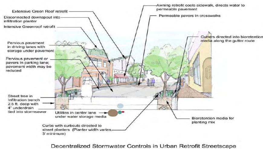
Figure 6.3.3 – Schematic example of engineered practices in an urban retrofit streetscape.
