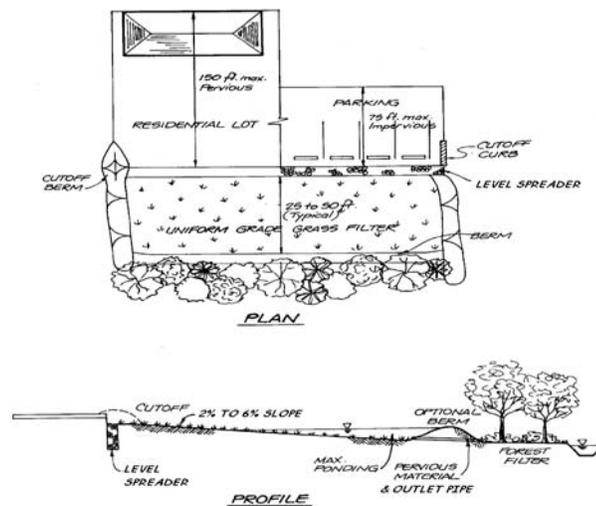
Figure 6.4.21 – Drawing of a vegetative filter strip. Source: Adapted from Atlanta Regional Commission, 2001.
