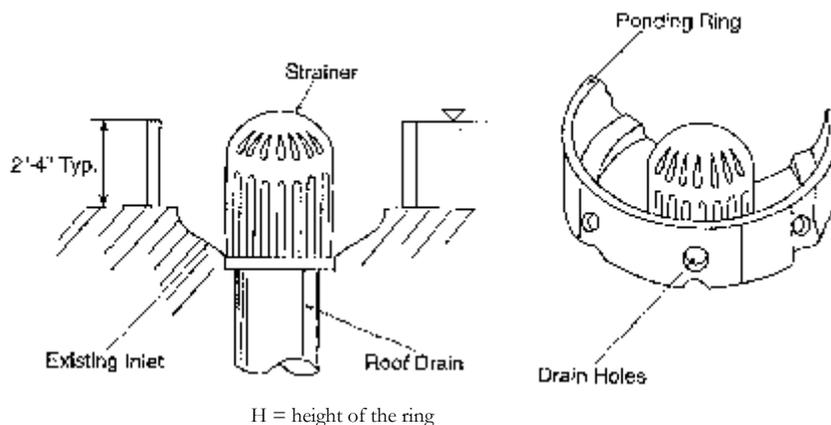
Figure 4.22 – Roof ponding rings. Source: Tourbier, 1974.
