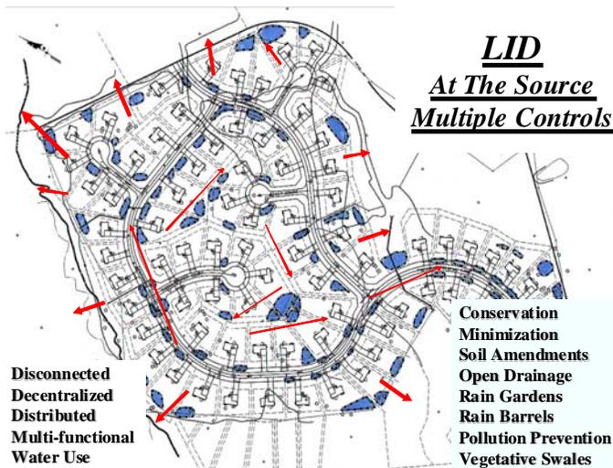
**Figure 2.2 – LID Controls.** A LID approach use a wide array of techniques that work with the landscape, soils, drainage patterns and vegetation to minimize impacts and integrated management controls to retain, detain, infiltrate and filter runoff. LID can provide better stormwater controls by mimicking the pre-development hydrology. Often LID designs increase lot yield and reduce infrastructure cost.
