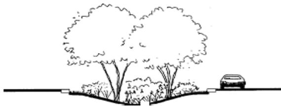
Figure 4.8 – Cul-de-sac infiltration island accepts stormwater from surrounding pavement. Note flat curb. Source: Connecticut, 2004.
