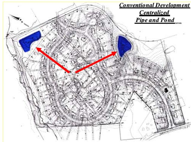
**Figure 2.1 – Conventional Controls.** A conventional approach requires clear cutting, mass grading and use impervious surfaces, gutters pipes and ponds to collect and treat runoff. This approach completely alters and destroys the natural hydrology and ability of the landscape to absorb rainwater and capture pollutants.
