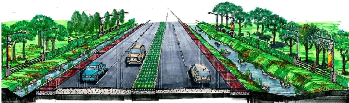
Figure 4.11 - Shoulder Treatment Systems using detention and filtration design.
