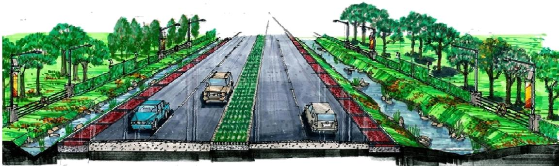
Figure 4.9 - Shoulder Treatment Systems using detention and filtration design.
