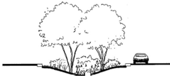
Figure 5.10 – Cul-de-sac infiltration island accepts stormwater from surrounding pavement. Note flat curb. Source: Adapted from Connecticut, 2004.
