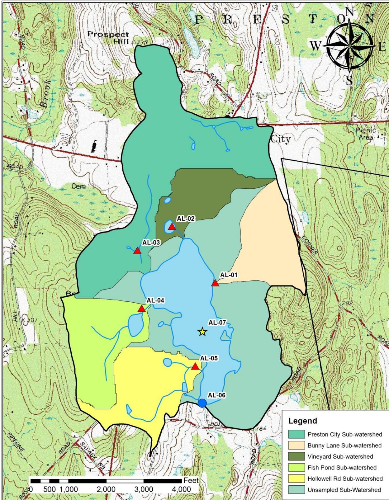
Figure 6-4. Delineation of sub-watersheds for pollutant loading estimations. Sampling sites are included for reference.
