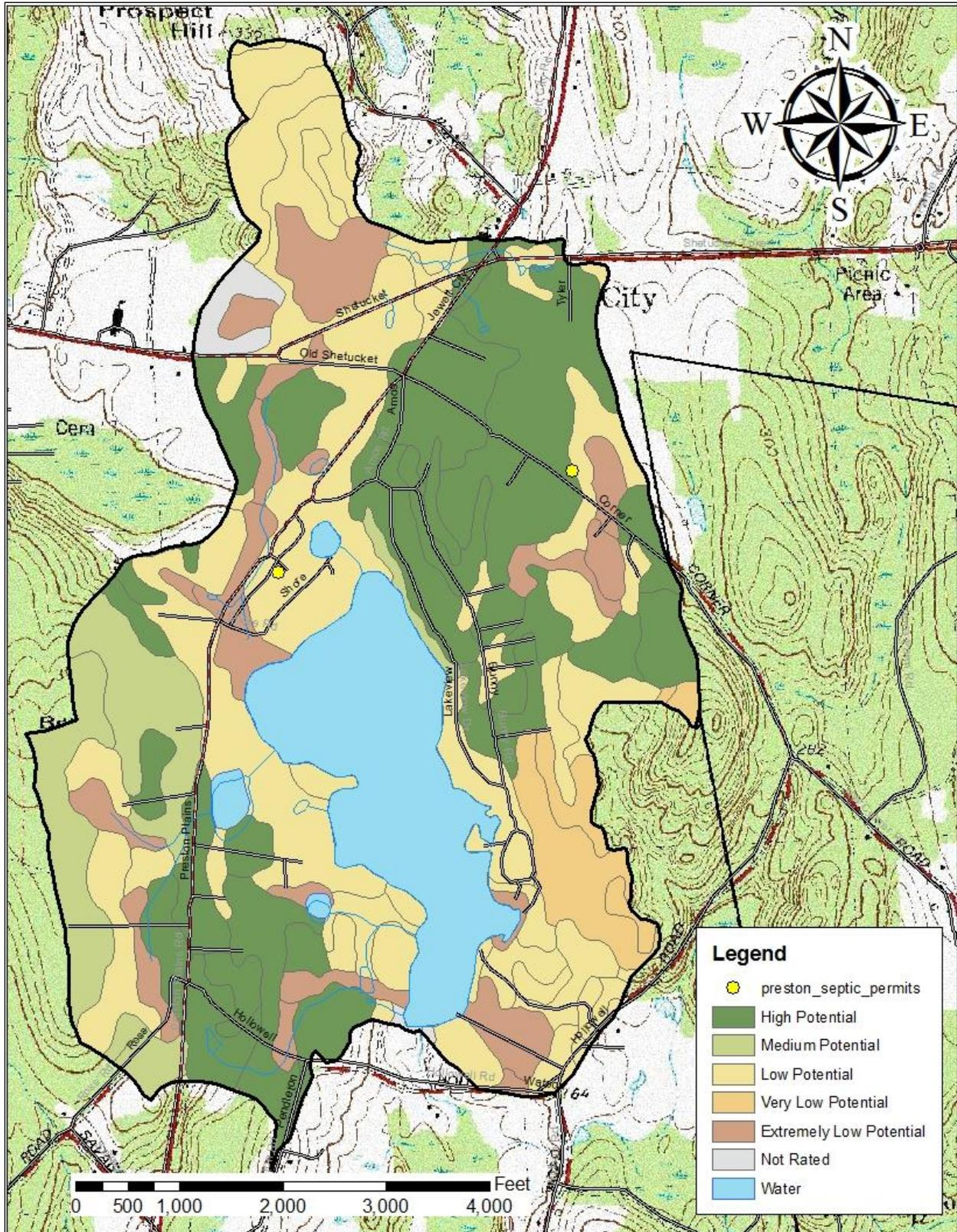
**Figure 5-2. Septic Suitability of soils in the Amos Lake watershed (USDA-NRCS Web Soil Survey) with locations of septic system repairs conducted between 2008 – 2013.**
