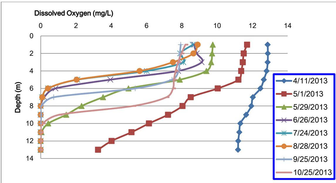
Figure 7 – Trend of anoxic boundary in Amos Lake during 2013
