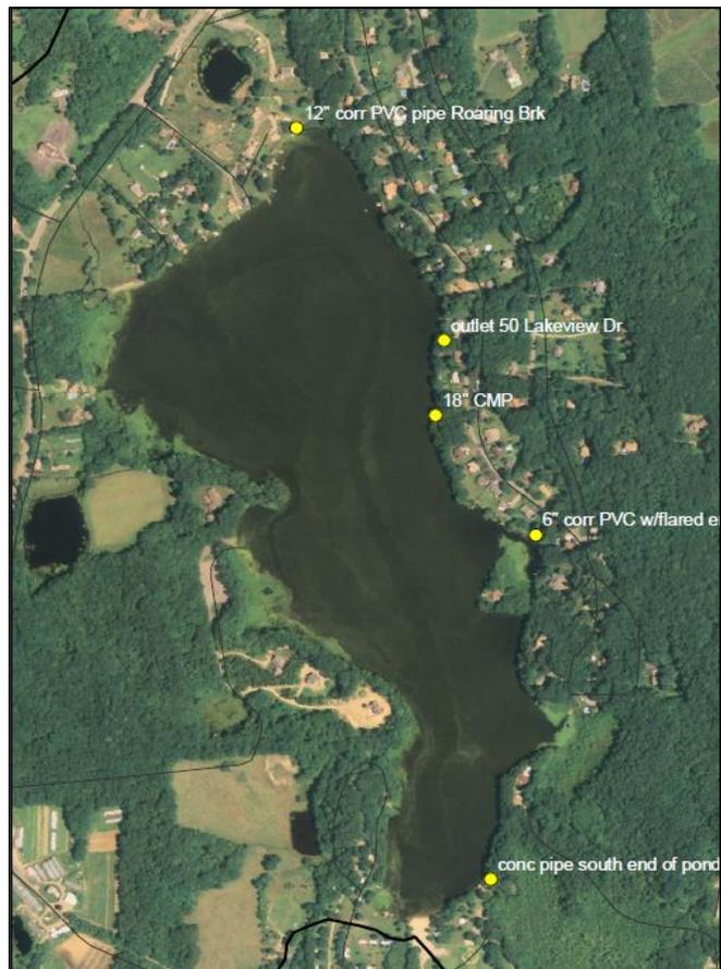
**Figure 5-4. Storm water outfalls to Amos Lake.**
