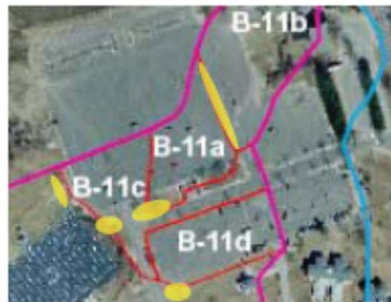
Figure 1. Location of proposed bioretention cells. Two portions of lot drain out of the Engleville Brook watershed (outside of pink line).
