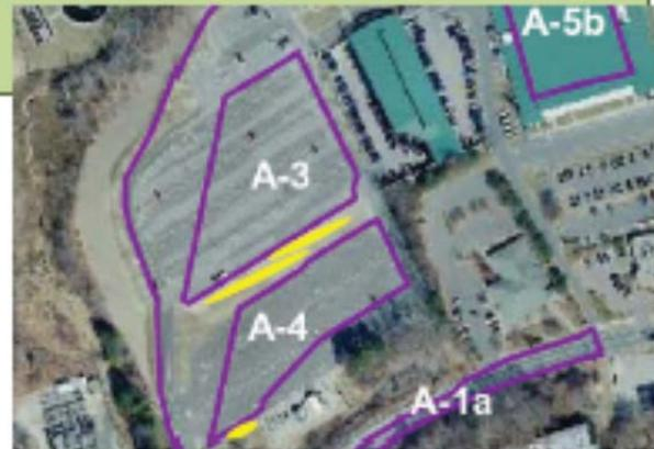
Figure 1. Drainage areas to proposed bioretention cells.
