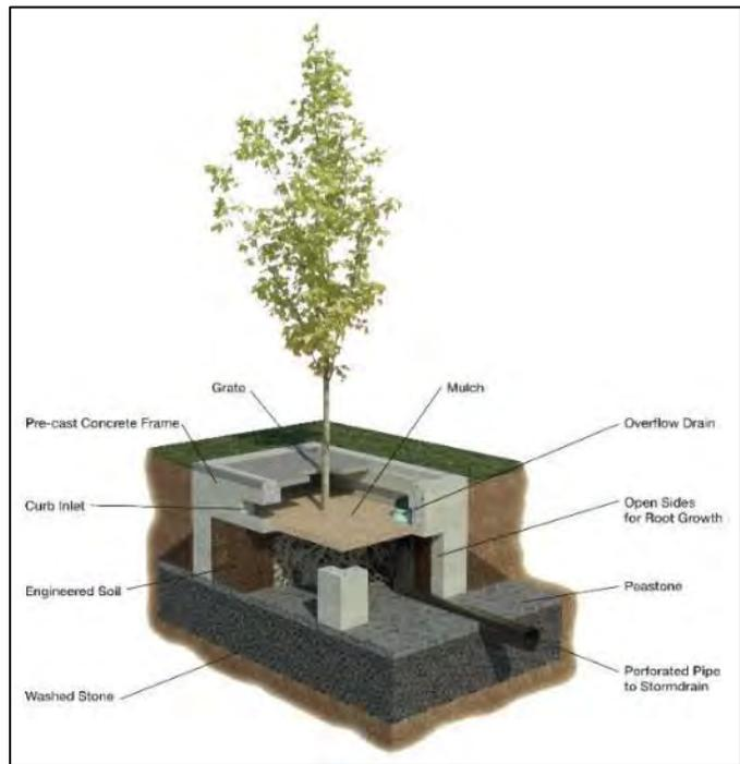
Figure 8-3. Schematic of a stormwater tree filter.
