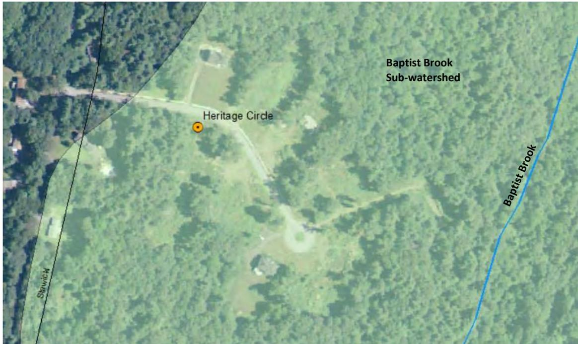
*Figure 8-2. Stormwater runoff from the Heritage Circle residential neighborhood is discharged near Baptist Brook, a Class A headwater stream that is part of the Thompson public drinking water supply watershed (Image USDA, 2012).*
