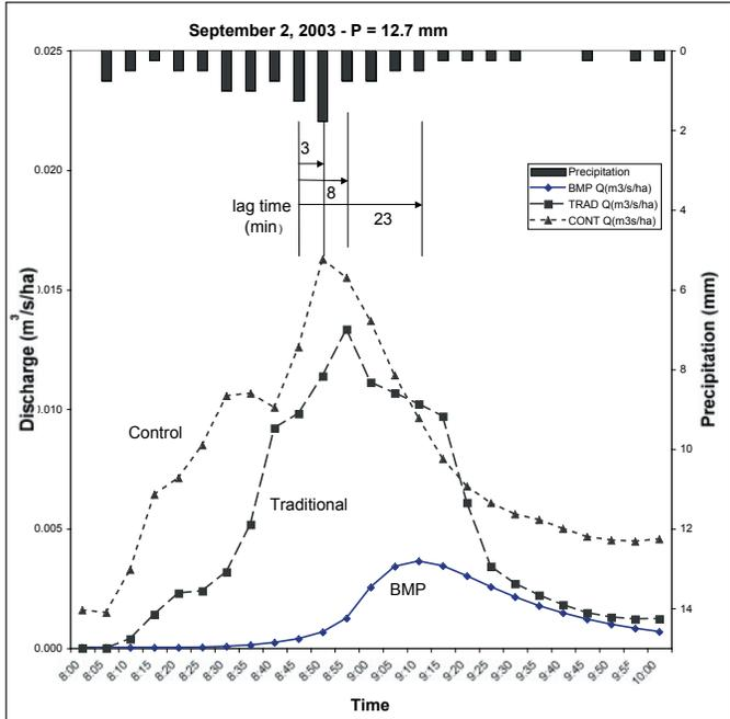
Runoff during this storm in 2003 showed a much lower peak and volume of runoff from the BMP watershed than from the others. The peak was delayed 15 minutes after the peak from the traditional watershed.
