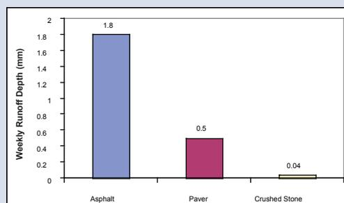
Runoff from the asphalt driveway was most, followed by the concrete paver driveway, and then the crushed stone driveway.
