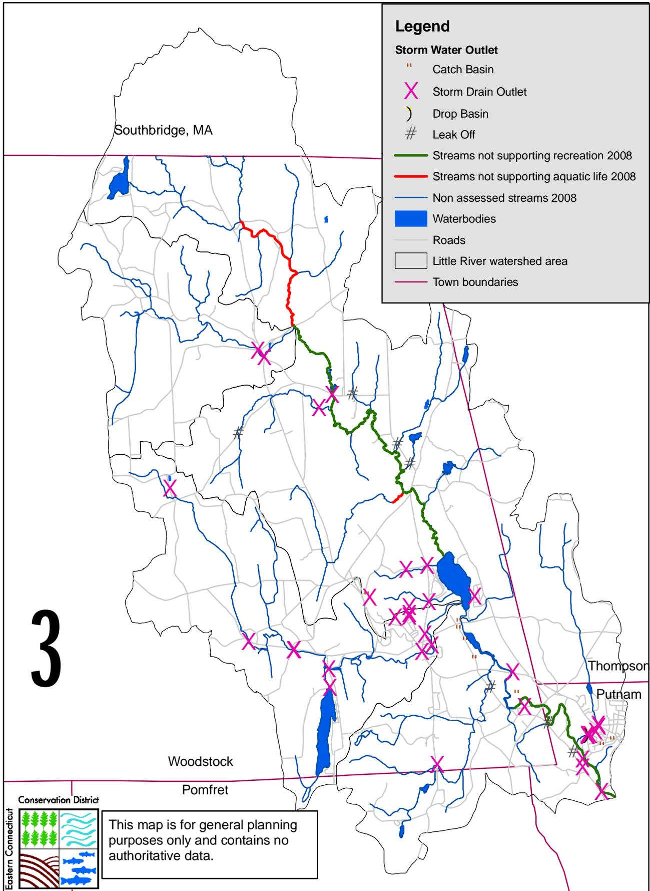
As part of the storm outlet survey, ECCD staff noted areas of concern (AoC) that related to the condition of the stormwater outlet area and potential pollutant contributions in the immediate vicinity, and other noteworthy issues. These AoCs are shown on Map 9, with further explanation in Table 4.
