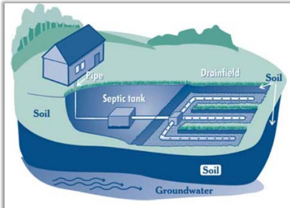
**Figure 5.1: Traditional septic system schematic. Source: USEPA**
