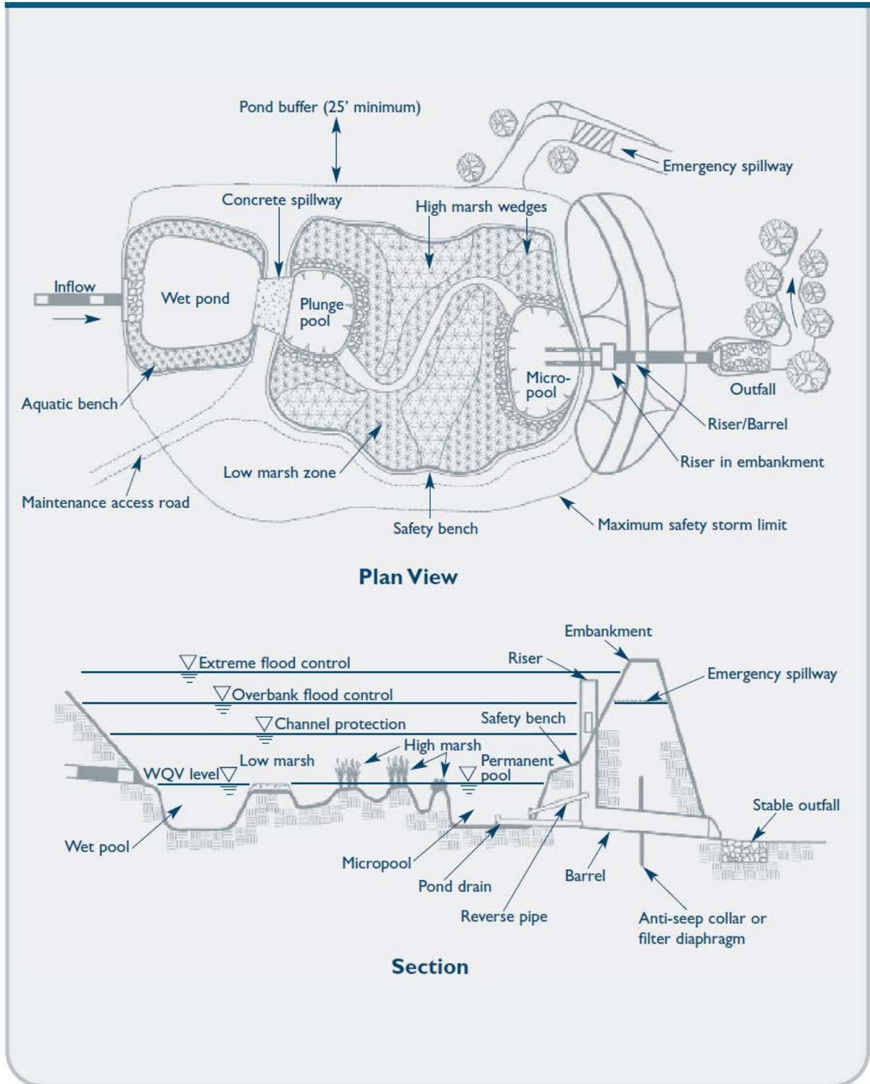
Figure 5.5: Pond/Wetland System. Source: CT Stormwater Quality Manual
