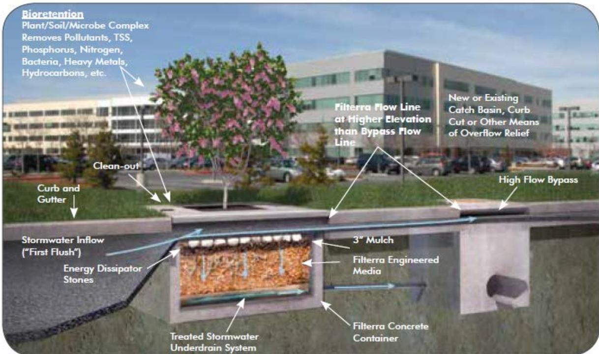
Figure 5.11: Tree Well Schematic. Source: Contech Engineered Solutions
