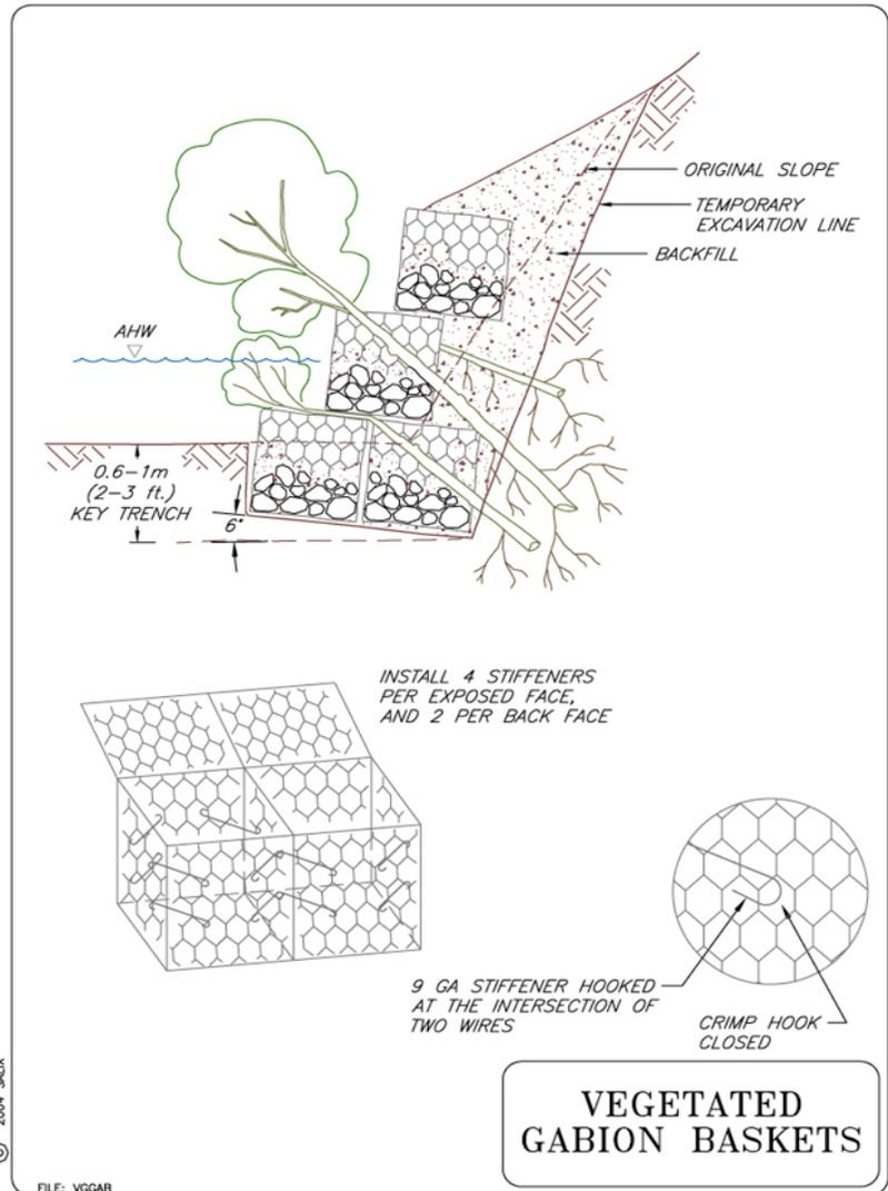
Figure 5.19: Gabion Detail
