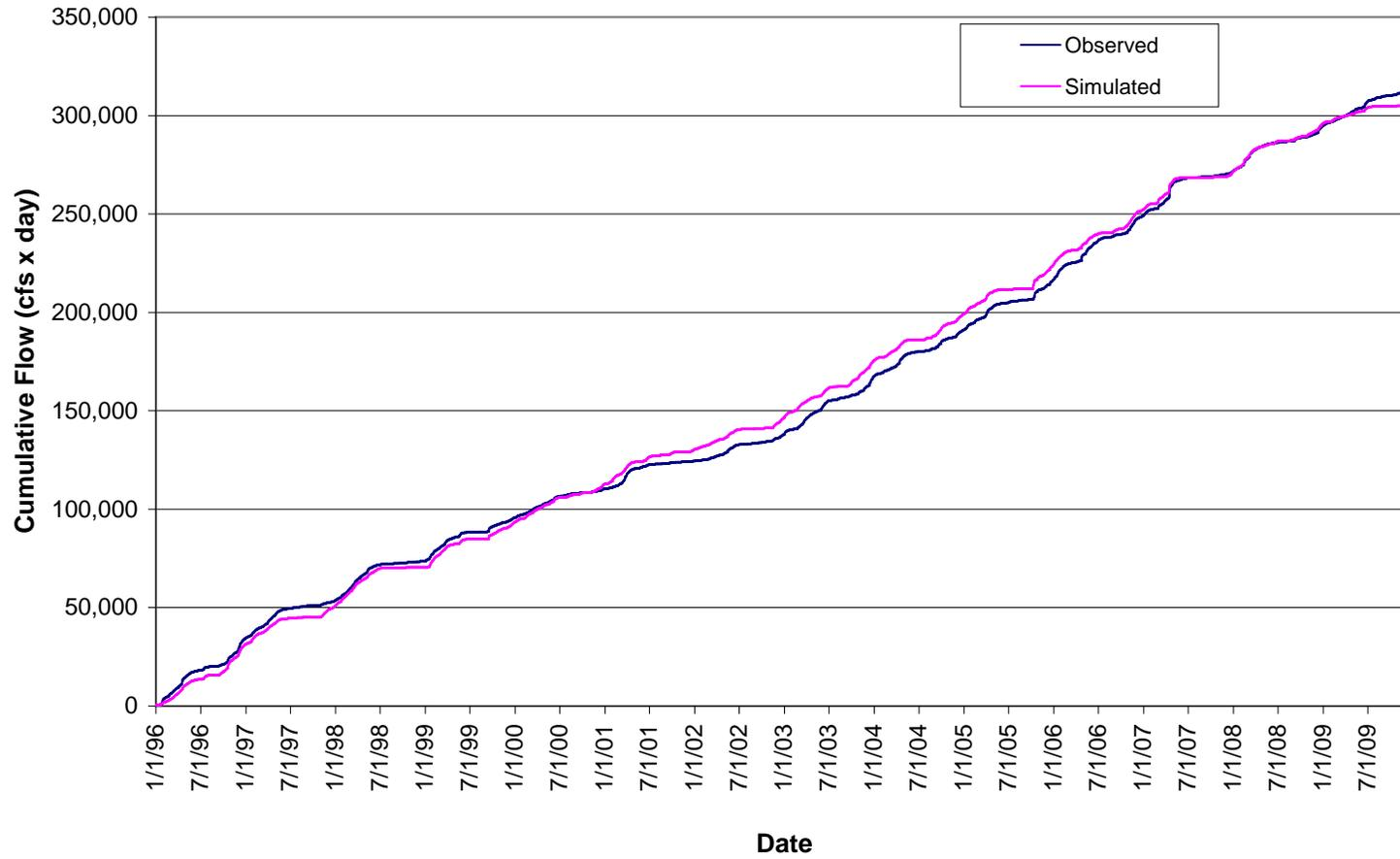
Figure C-7. Cumulative flow comparison at South Wilton (1996-2009)
