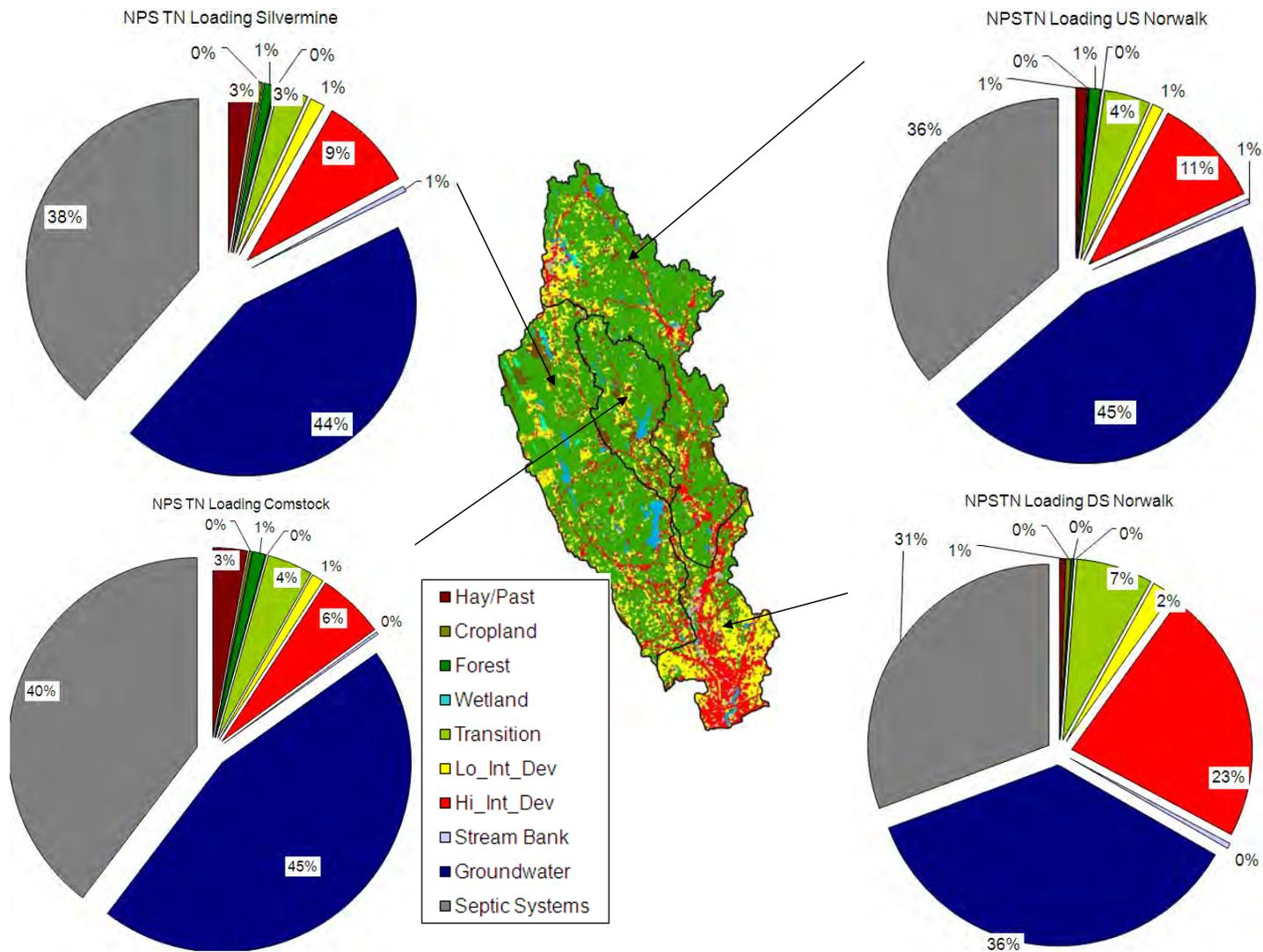
Figure C-11. Calculated TN Loads from Various Non-point Pollution Sources
