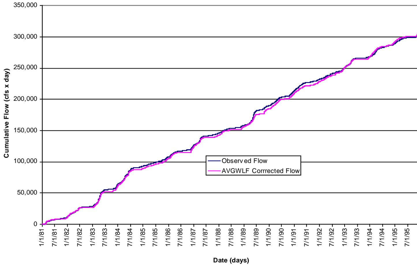
Figure C-5. Cumulative flow comparison at South Wilton (1981-1995)
