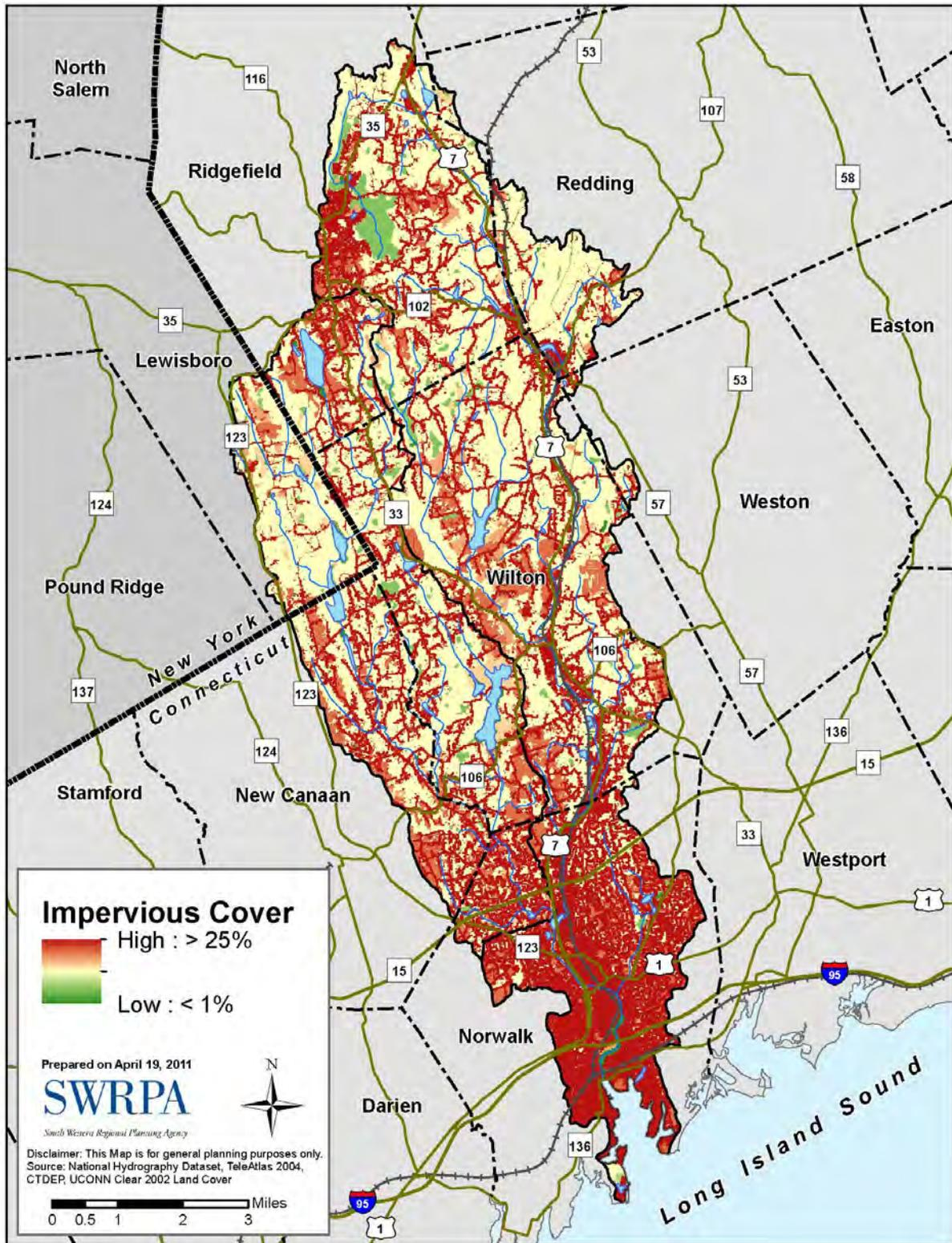
Figure 3-4. Watershed Impervious Cover
