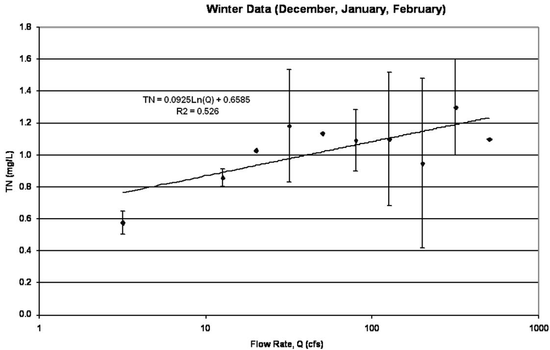
**Figure C-8. Relationships between TN and flow rate for (a) spring, (b) summer, (c) fall, and (d) winter.**
