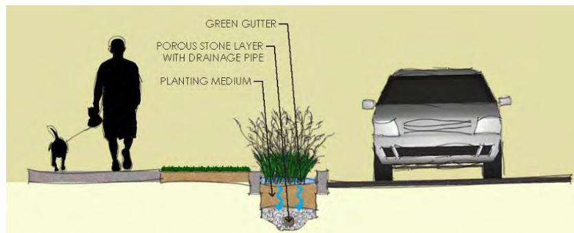
**Figure 4-9. Typical Green Gutter Cross Section**
