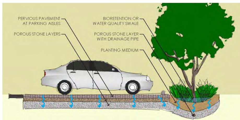
**Figure 4-10. Typical Pervious Parking Row Cross Section**
