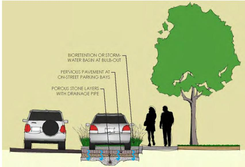
Figure 4-17. Typical Pervious Pavement Parking Stall
