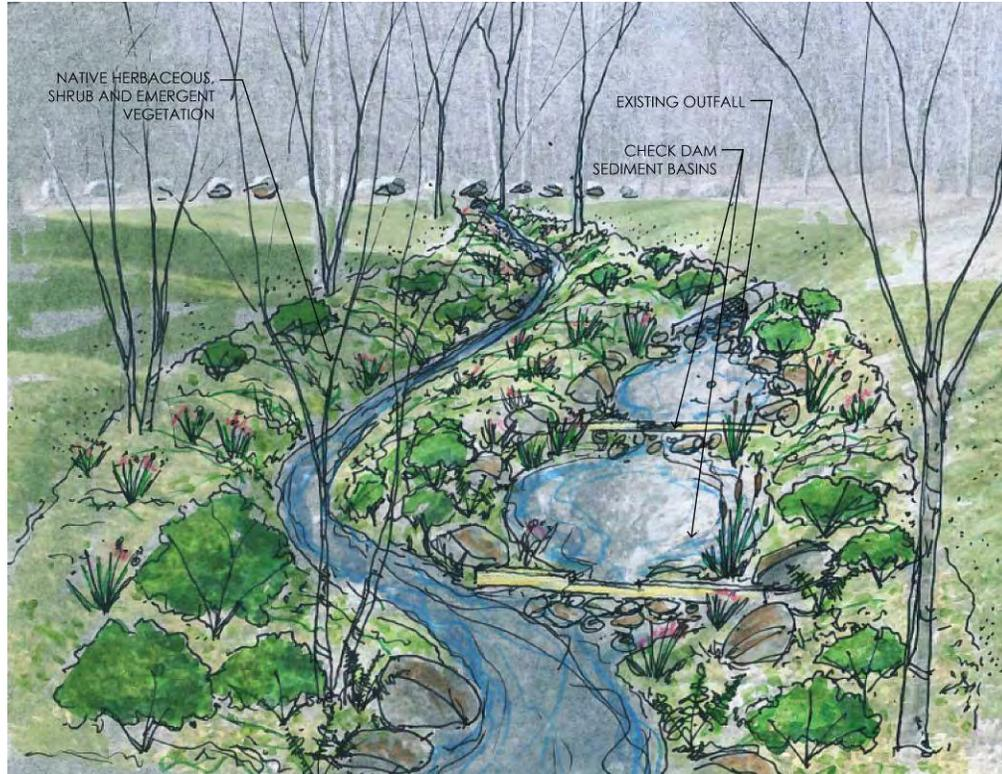
**Figure 4-3. Proposed Stream Restoration Concept**
