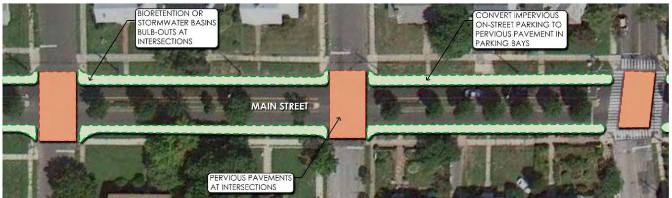
Figure 4-18. Green/Complete Street Concept Site Plan
