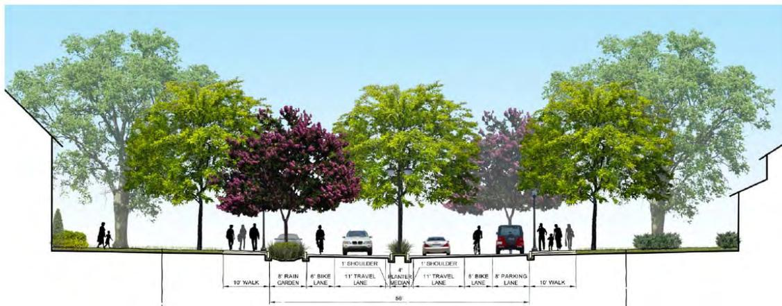
**Figure 4-20. Green/Complete Street Cross Section**
