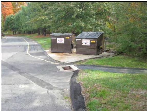
Runoff or leaking from these dumpsters would drain to the stormwater drainage system.
