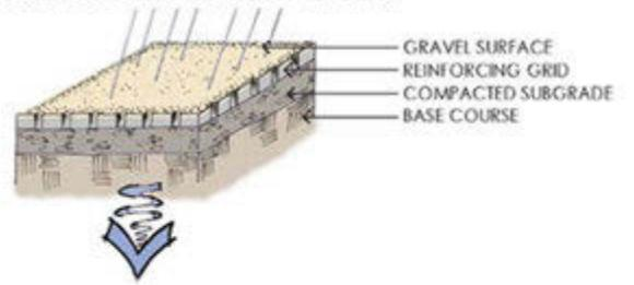
**PERVIOUS JOINT PAVEMENT DIAGRAM**
