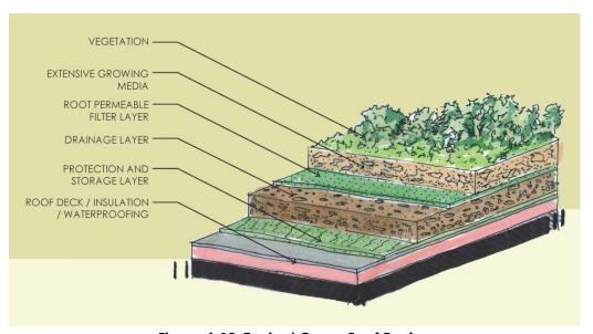
Figure 4-10. Typical Green Roof Design
