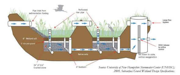
Figure 4-17. Typical Subsurface Gravel Wetland Design
