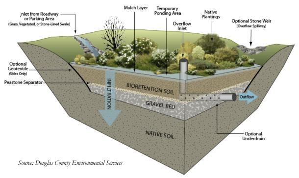
Figure 4-5. Typical Bioretention Design
