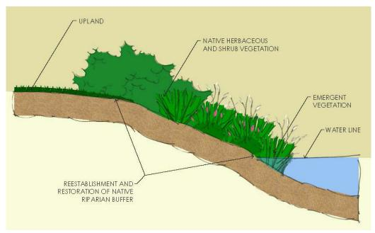
Figure 4-21. Typical Bank Restoration Planting for Small Streams
