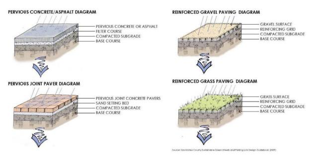
Figure 4-13. Diagrams of Selected Permeable Pavement Systems
