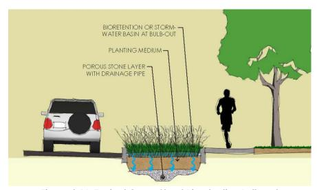
Figure 4-16. Typical Green Street Bioretention Bulb-out
