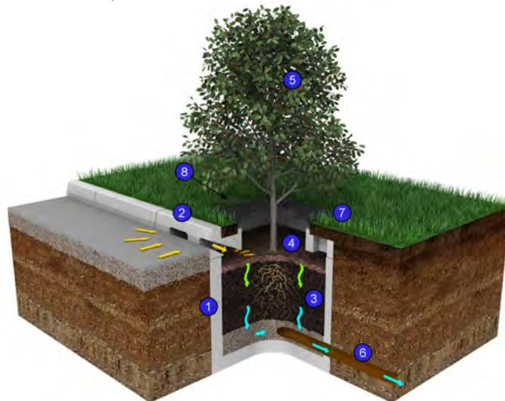
Figure 2.2.2. Typical Tree Box Filter (Source: Hydro International, Inc.)
