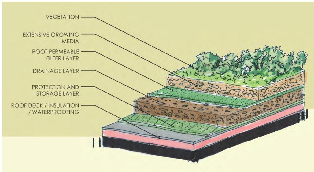
Figure 2.2.4. Typical Green Roof Design
