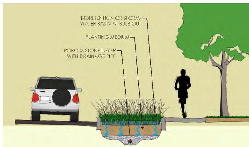
**Figure 2.4.3. Typical Green Street Bioretention Bulb-out**
