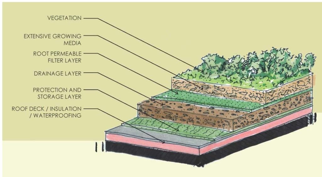
**Figure 4-7. Typical Green Roof Design**
