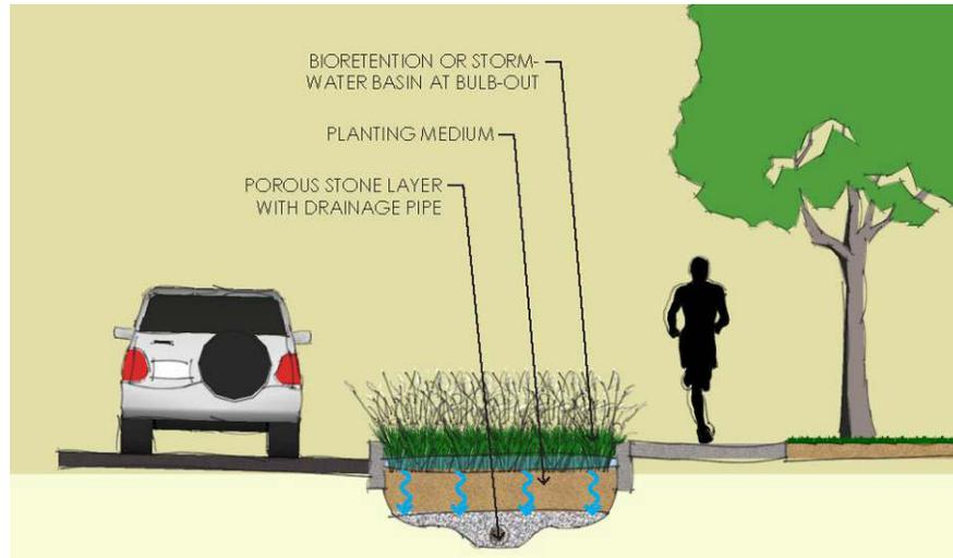
Figure 4-22. Typical Bioretention Bulb-out
