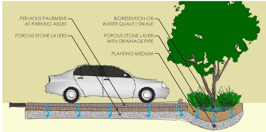
**Figure 4-3. Typical Pervious Parking Stalls with Vegetated Swale**
