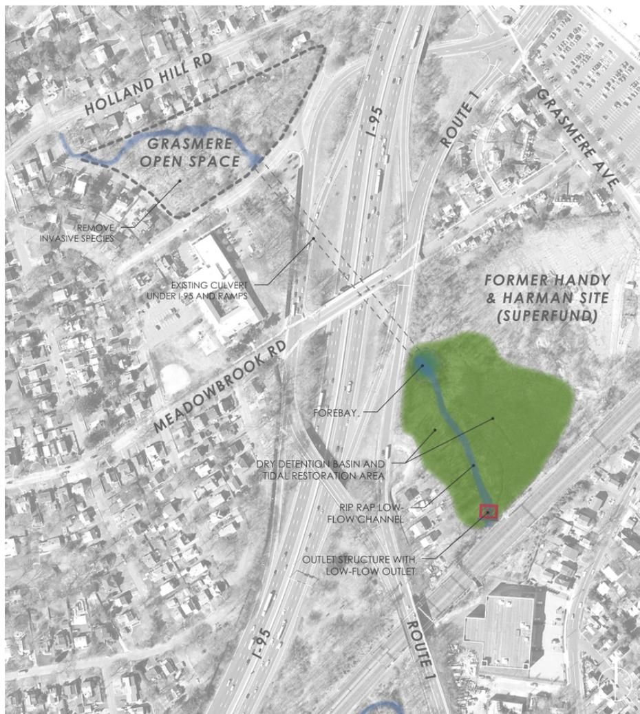
**Figure 9. Flood Storage and Tidal Wetland Restoration at the Former Handy & Harman Site**
