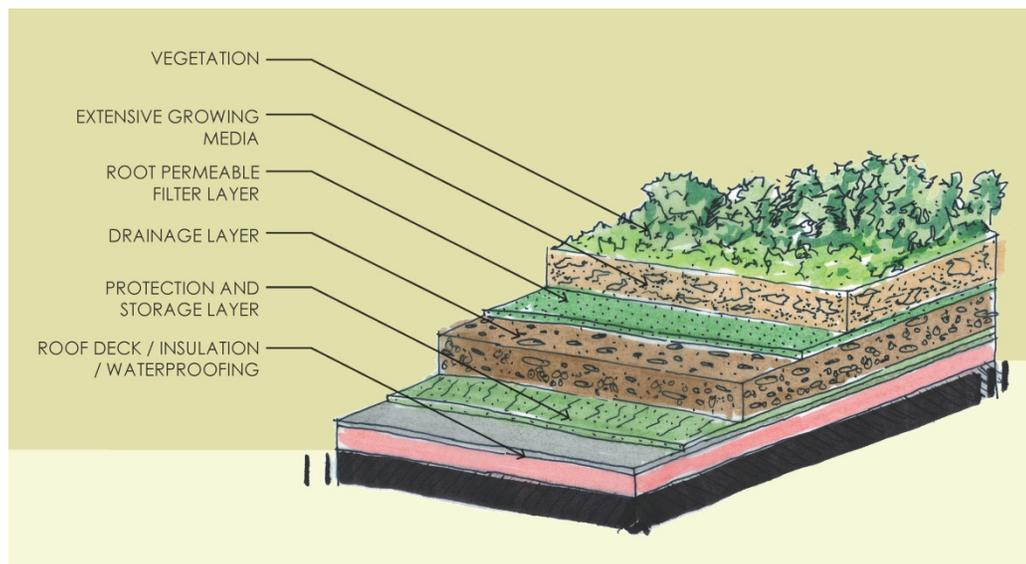
**Figure 6. Typical Green Roof Design**
