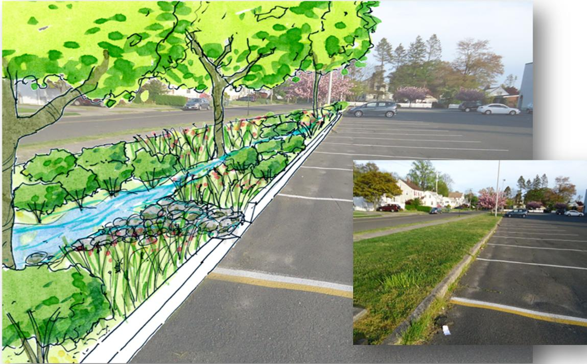
**Figure 7. Before and After Concept Design for a Bioretention Area for the Parking Lot**
