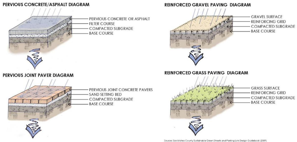
**Figure 8. Diagrams of Selected Permeable Pavement Systems**
