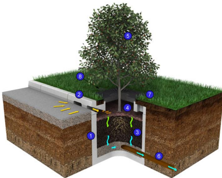
**Figure 14. Typical Tree Box Filter (Source: Hydro International, Inc.)**
