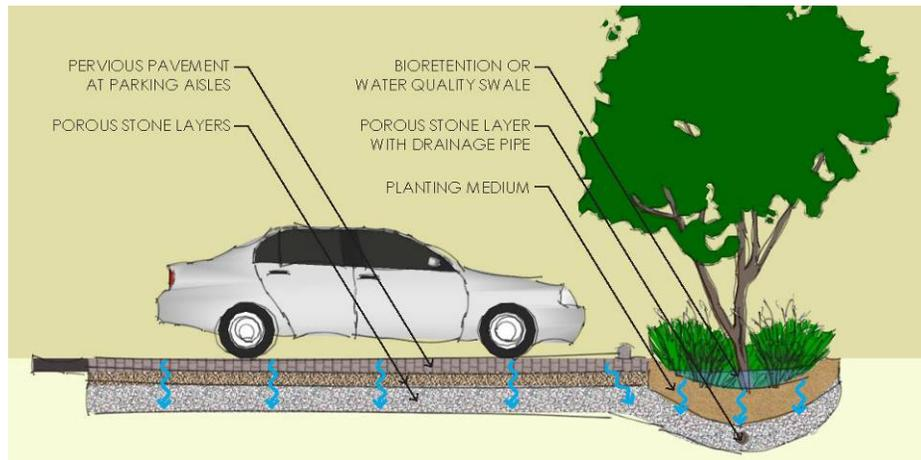
**Figure 2. Typical Pervious Parking Stalls with Vegetated Swale**
