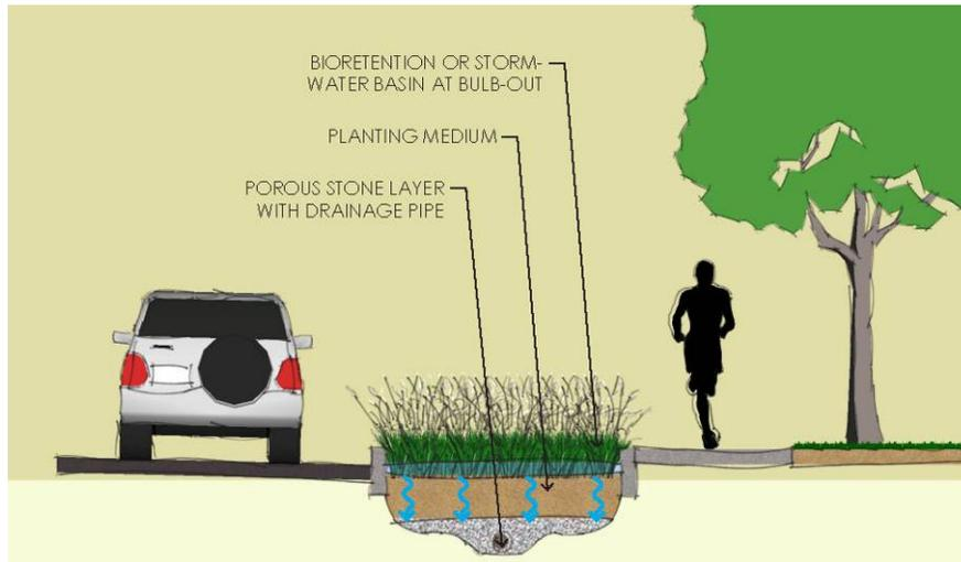
**Figure 21. Typical Bioretention Bulb-out**
