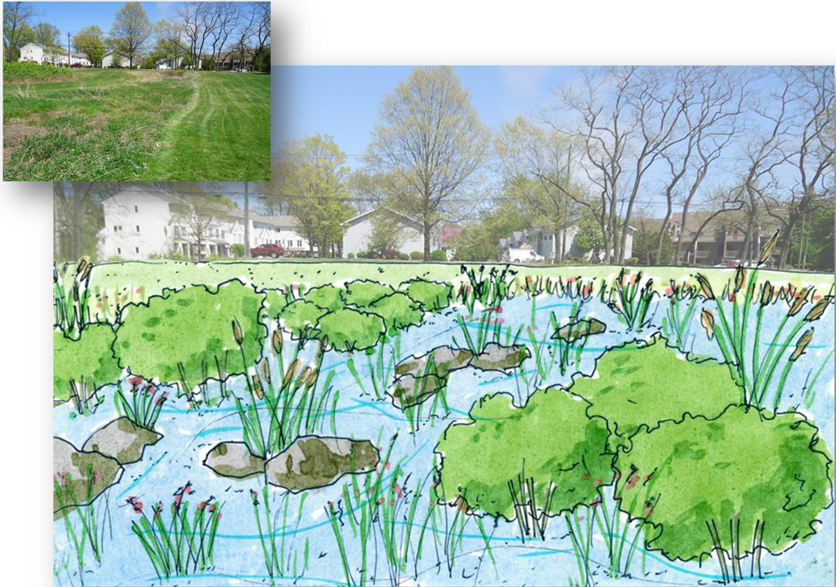
**Figure 15. Existing and Proposed Bioretention Basin at the Bridgeport Public Library**
