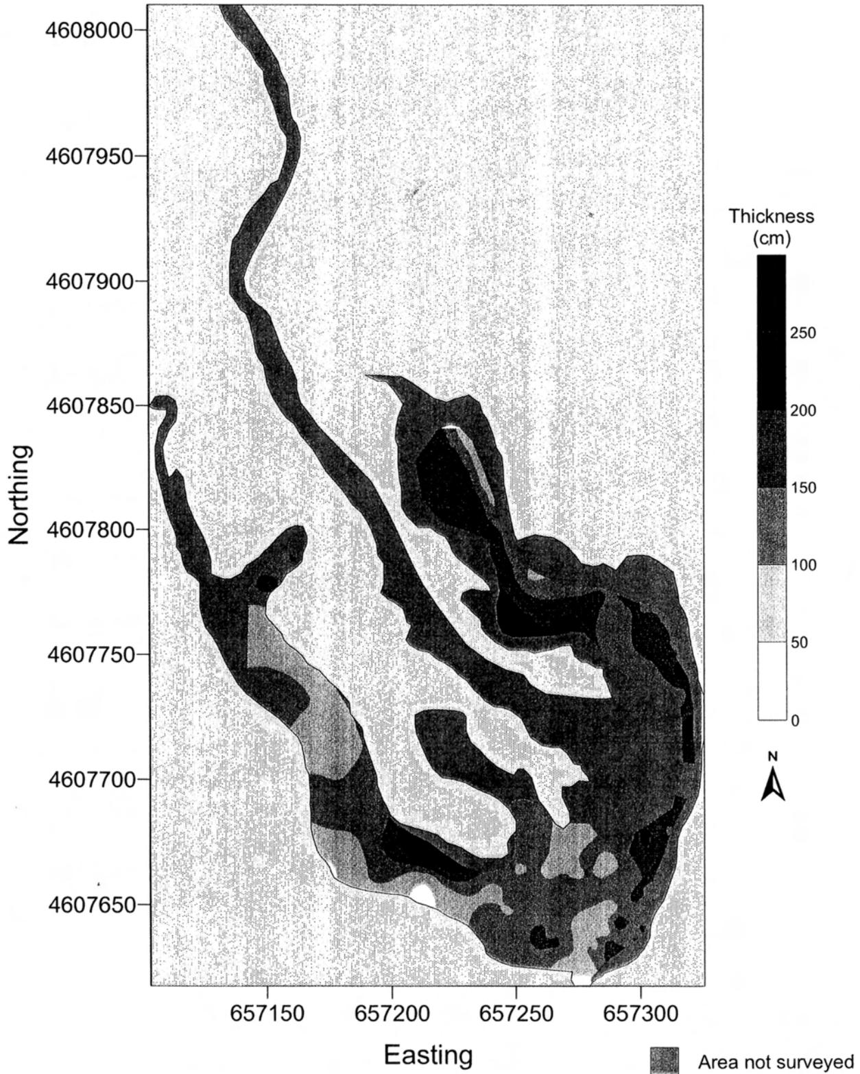
Figure 5. GPR interpreted thickness of bottom sediments within Hemingway Pond. The extensive areas shown in green were not surveyed because they were too shallow or too overgrown with vegetation.
