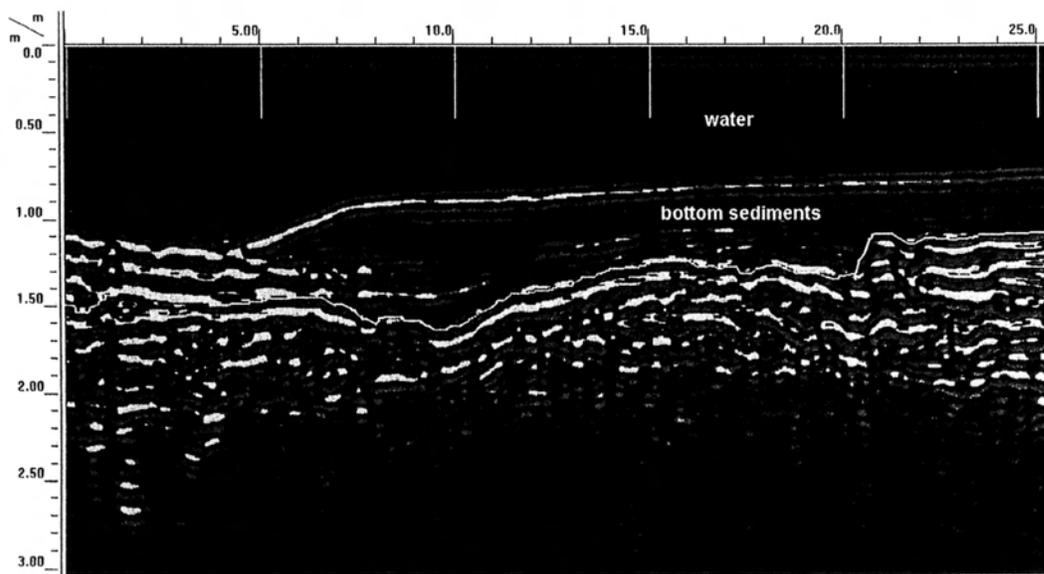
Figure 2. Each material has dissimilar dielectric properties and unique graphic signatures on this portion of a radar record from Hemingway Pond.
