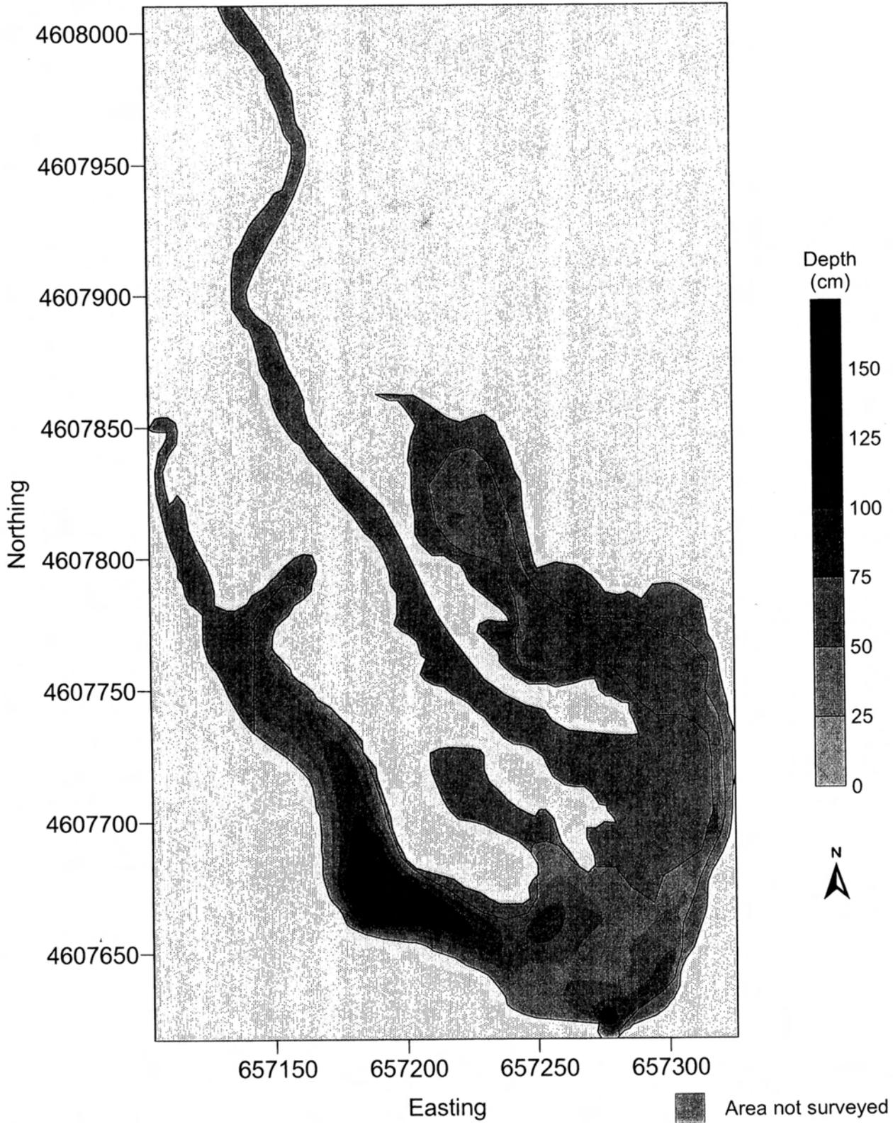
Figure 4. GPR interpreted depths of water within Hemingway Pond. The extensive areas shown in green were not surveyed because they were too shallow or too overgrown with vegetation.
