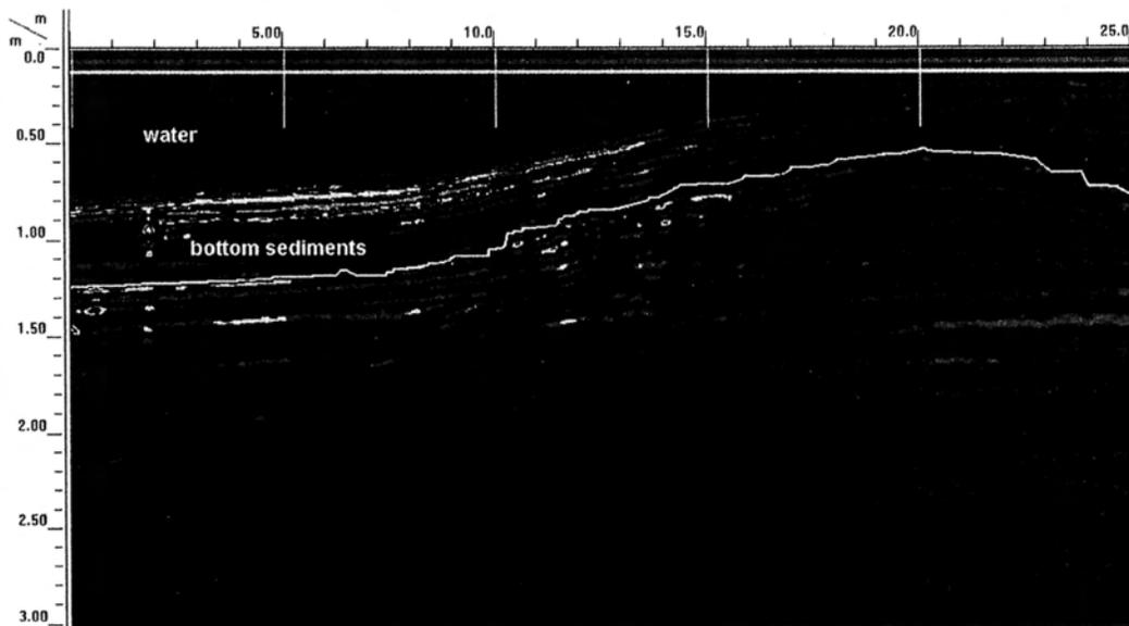
Figure 3. In some portions of Hemingway Pond interfaces are too closely spaced, gradational, or separate less dissimilar materials and are difficult to interpret.
