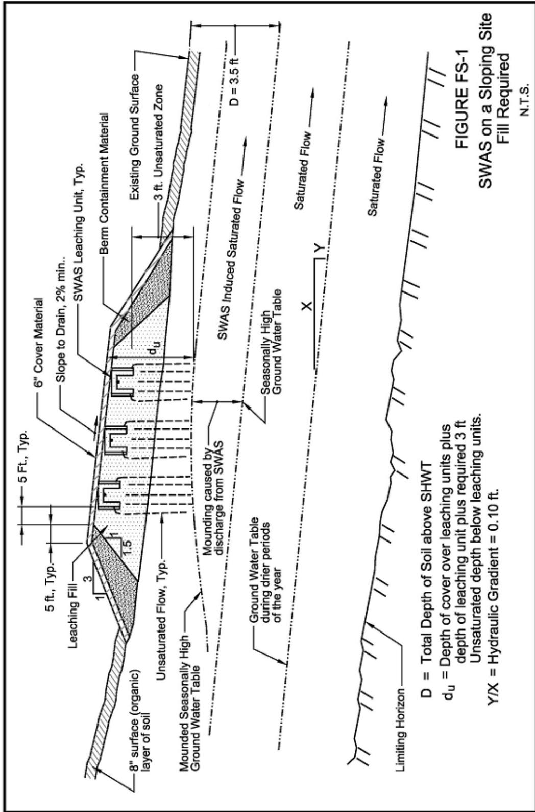
Hydraulic analyses for determining the thickness and lateral dimensions of the fill will differ in detail and complexity depending upon the nature and configuration of the system. A number of variables have to be considered in the design of a LSF, including:
