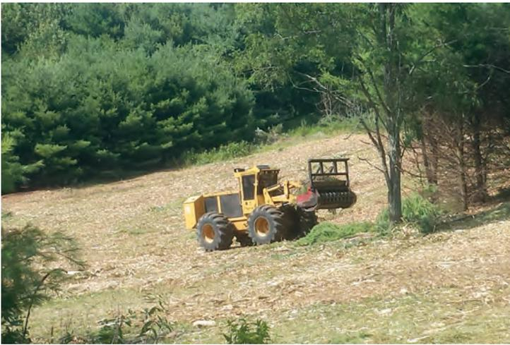
Skidder with front-mounted mower removing white pine and autumn olive.
