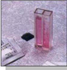
**Colorimetric tests** use a reagent which changes color depending on the concentration of the chemical being tested. The color is then compared to a standard to determine the concentration. Disinfectant and pH are usually tested using this method.
