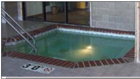
**SPA POOL DECK EXCEPTION** - A spa pool must have a minimum of 4 feet of unobstructed decking around at least 50% of the spa. Half of the perimeter of a spa may be next to a wall, fence or guard rail if this portion of decking is one (1) foot or less in width.
