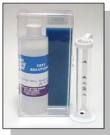
**Turbidimetric tests** measure the amount of suspended solids in the water. The sample becomes cloudier in proportion to the concentration of the chemical being tested. This test is used to measure the level of cyanuric acid (stabilizer) in the water.
