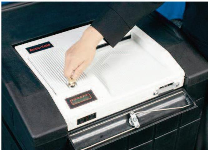
Step 16 – Replace and lock the printer cover
