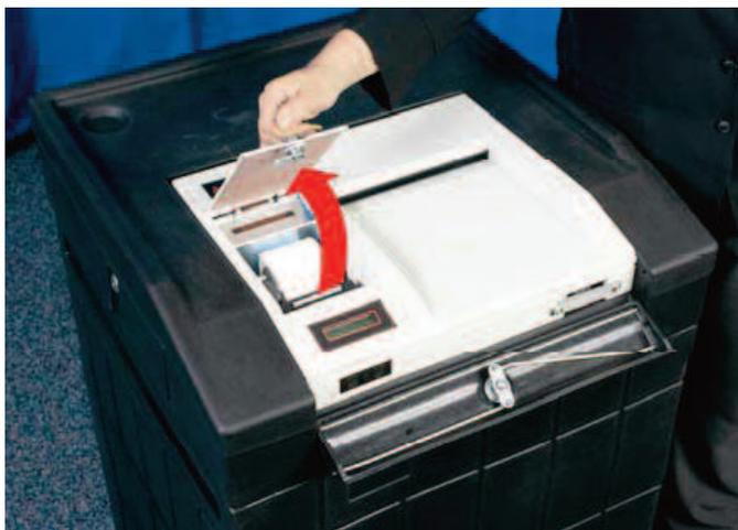
Step 8 – Unlock and remove printer cover
