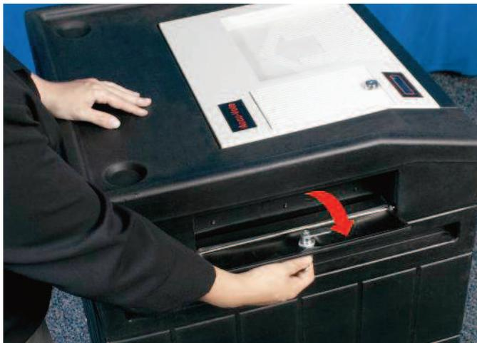
Step 21 – Unlock and open Auxiliary Slot
