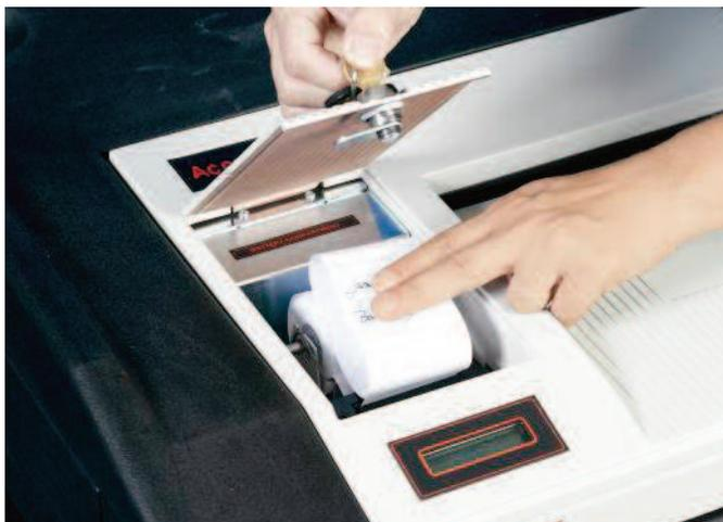
Step 17 – Fold up third copy of tape and replace printer cover
