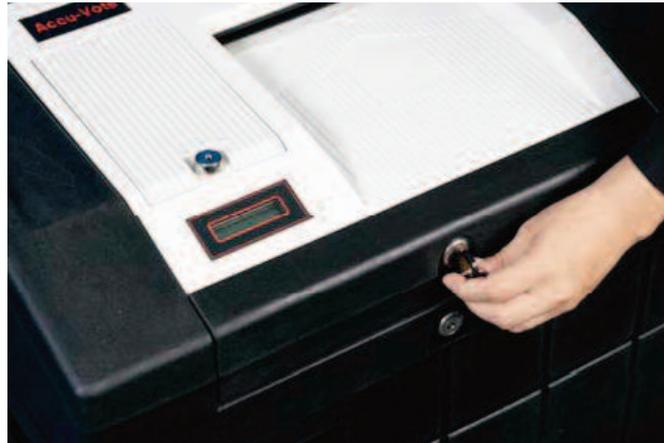
Step 1 – Unlock and open retaining door
