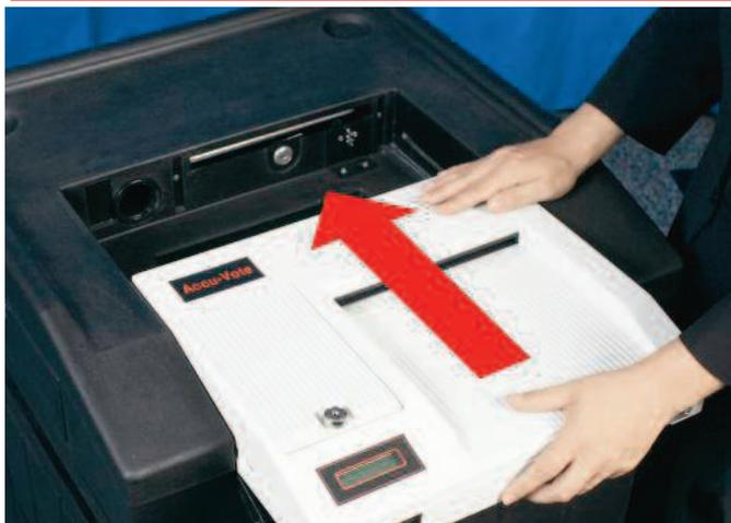
Step 8 – Slide the Optical Scan halfway into the ballot box
