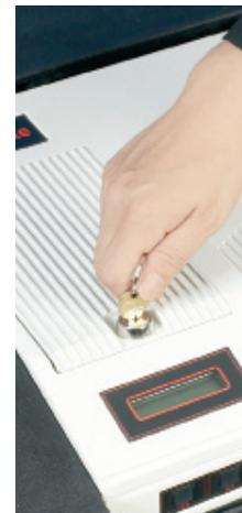
4 Unlock and remove the printer cover using the plain brass key. Unlock and open the retaining door of the ballot box using the brass key with plastic key cap.
