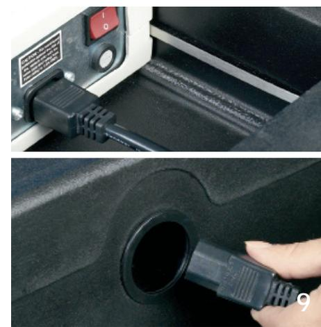
9 Turn off the AccuVote unit by pressing the red ON/OFF switch on the back of the unit. Unplug the power cord from the UPS unit, unplug the unit and remove the power cord. Repack the unit in its case.
