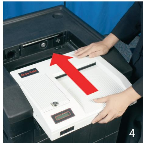
Remove the AccuVote unit from its carrying case and guide the unit into position on top of the ballot box. Be sure to leave enough space between the unit and the ballot box to reach the red ON/OFF switch on the back of the unit.
