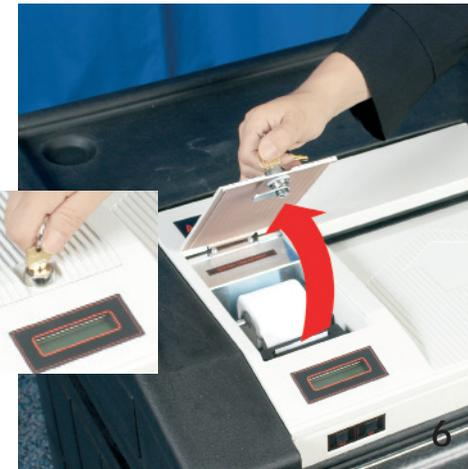
Using the plain brass key, unlock and remove the printer cover. Place it on the back of the ballot box.
