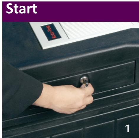
1 After the last voter has cast their ballot, lock the auxilliary on the left side of the ballot box and unlock the lower door using the key with the plastic cap.
