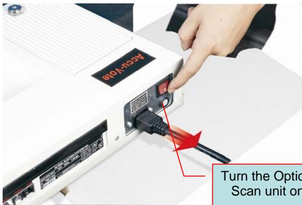
Turn the Optical Scan unit on
