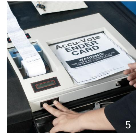
5 Locate the ENDER Card. Press and hold the YES and NO buttons at the same time. While holding the two buttons, insert the ENDER CARD into the AccuVote unit.
