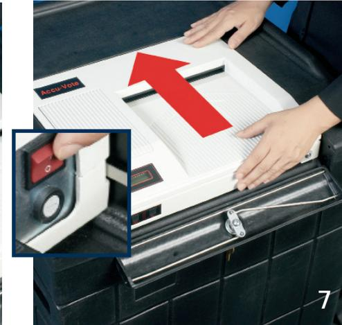
Power the AccuVote unit on by pushing the red ON/OFF switch on the back of the unit and then finish sliding the unit firmly into place.
