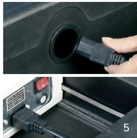
Thread the power cord through the power cord tunnel on the back of the ballot box and connect to the AccuVote unit. Plug the power cord into the UPS unit. Plug the UPS unit into the wall.
