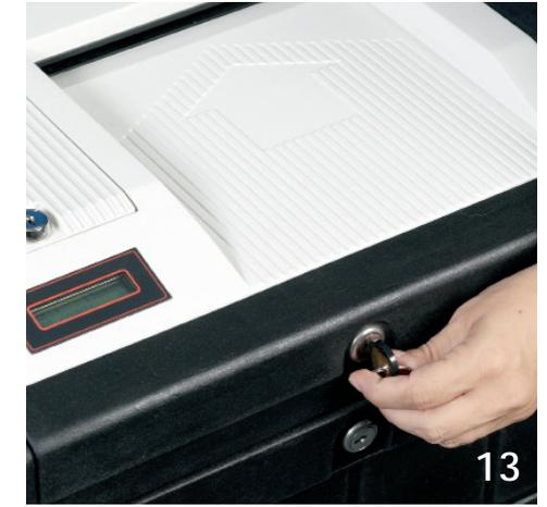
13 Lock the retaining door on the ballot box using the key with plastic cap.
